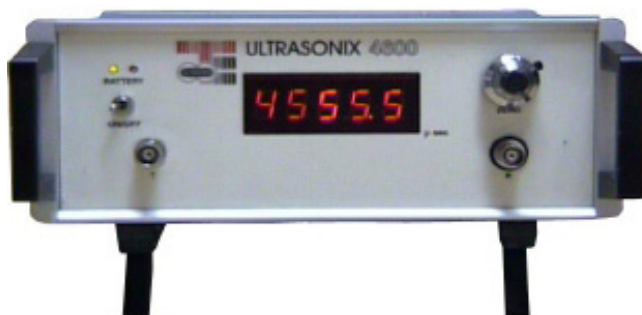
Fig. 6. Compressional wave velocity (P-wave) measuring device 'Ultrasonix 4600'
