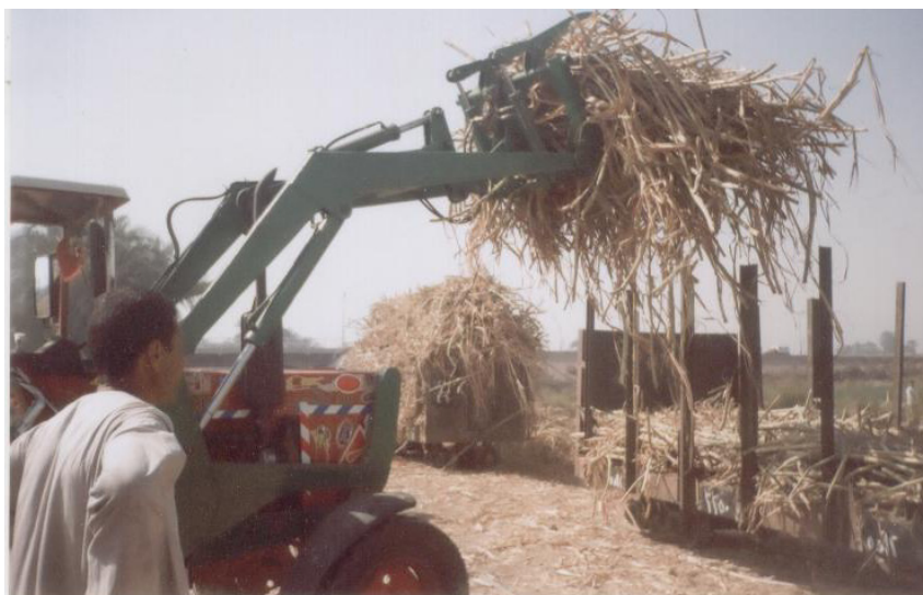
Fig. 13. Mechanical loading of light railway wagons using a tractor mounted loader (developed by the author).
