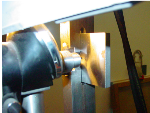
Fig. 14. Experimental tests in order to establish the material constants C and m
