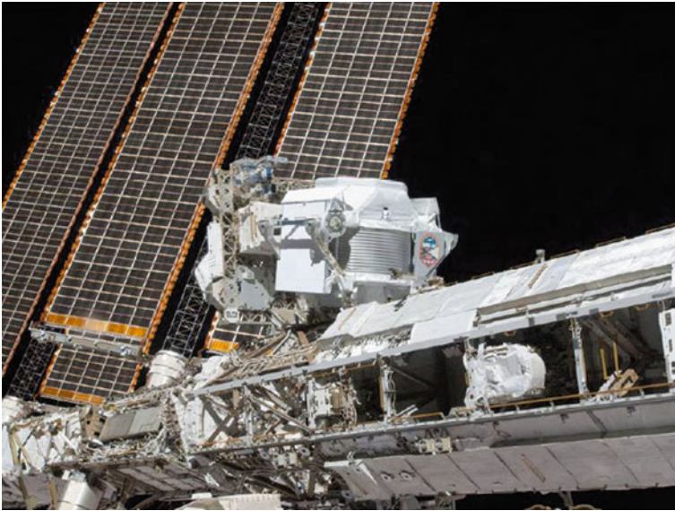
Fig. 1.6 The Alpha Magnetic Spectrometer (AMS) detector on-board of the International Space Station (Photo: courtesy AMS-02 Collaboration)
