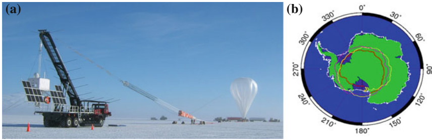
Fig. 3.2 a CREAM ballooncraft with the launch vehicle while a 10^6 \text{ m}^3 balloon is being inflated at the launch site, Williams field near McMurdo, Antarctica; b the balloon trajectory of a 37 day flight of CREAM, which was launched on December 1, 2009 and terminated on January 8, 2010 during about three rounds of the South Pole. Courtesy of Prof. E. Seo (CREAM Collaboration) ( http://cosmicray.umd.edu/cream/ )
