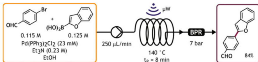
Scheme 17 Suzuki-Miyaura coupling under microwave irradiation directly transferred from batch to flow (Wilson et al. [49])
