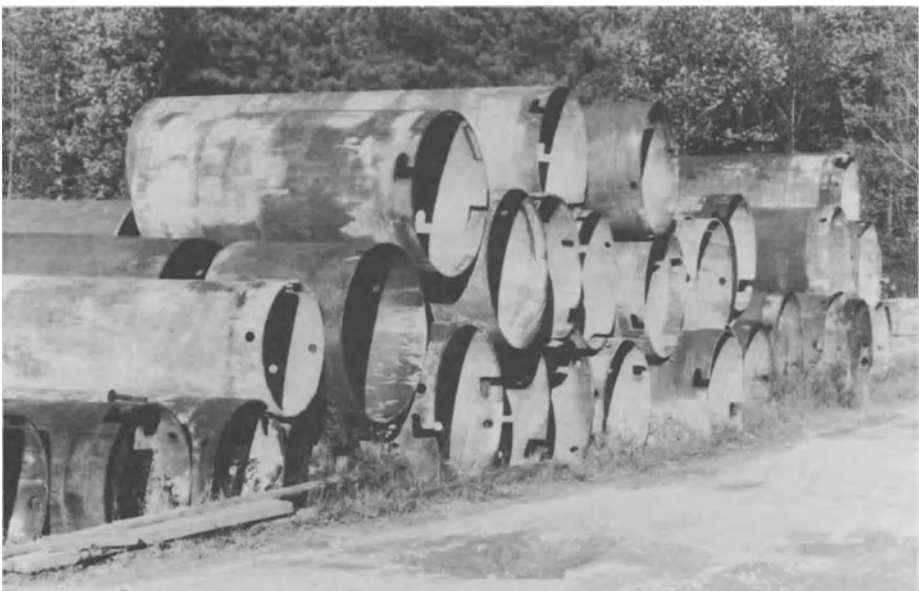
FIGURE 6-10. Steel liners, used in caisson installation to prevent side wall collapse and to protect workmen. [Ref. 14]
