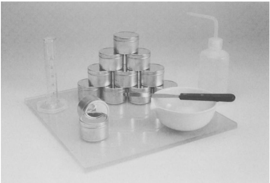
FIGURE 11-3. Plastic limit testing set. [Ref. 4]
