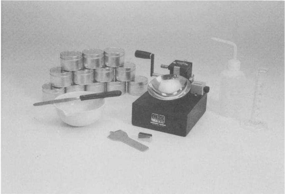
FIGURE 11-2. Liquid limit testing set. [Ref. 4]
