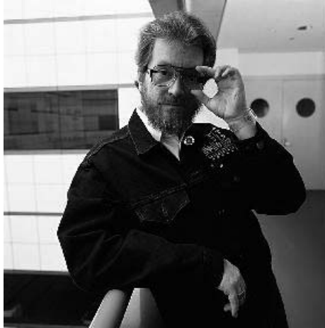
Figure 15.9 The author wearing a variety of new technologies. The glasses (built by Microoptical of Boston) contain a computer display that is nearly invisible to others. The jacket has a keyboard that is literally embroidered into the cloth. The lapel has a “context sensor” that can classify the user’s surroundings and, of course, there is a computer that is not visible in this photograph. Photo by Sam Ogden.
