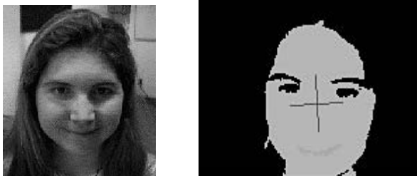
Figure 15.7 The LAFTER system finds and tracks face and facial features at 30 Hz, feeding facial feature geometry for HMM expression recognition.
