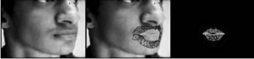
Figure 15.8 Fitting a 3-D FEM to facial data, allowing us to extract pose-invariant 3-D lip shape.
