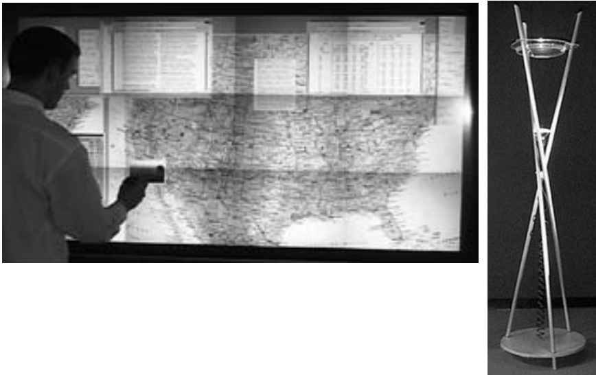
Figure 7.3 The figure on the left is the Stanford Interactive Mural, an example of a large-scale interactive display surface created by tiling multiple lower-resolution projectors. Picture courtesy of Françoise Guimbertière. The figure on the right is an example of an ambient display, the Water Lamp, from Ishii's Tangible Media Group at the MIT Media Laboratory. Light shines up through a pan of water, actuated by digitally controlled solenoid that can tap the water and cause ripples. External information can be used to drive the tapping of the solenoids. Picture courtesy of Hiroshi Ishii.
