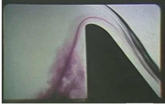
Fig. 3.11 Curvilinear flow over spillway, after Rouse (IIHR movie Fluid motion in a gravitational field)
