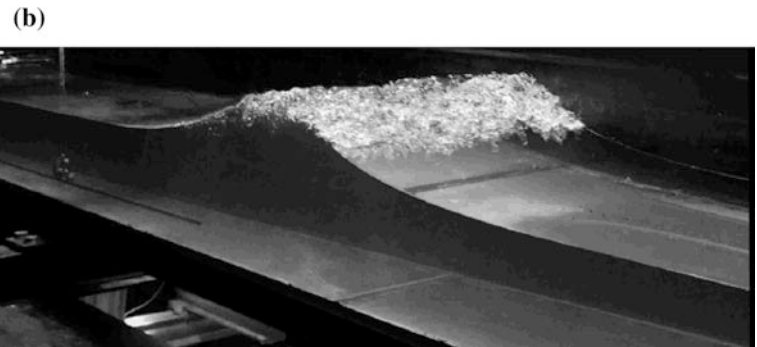
Fig. 5.46 Solitary wave a original drawing after Boussinesq (1877), b wave breaking (Photograph VAW)
