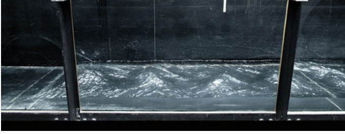
Fig. 2.7 Undular hydraulic jump. Note the highly 3D free surface flow pattern (photograph VAW, ETH Zurich)
