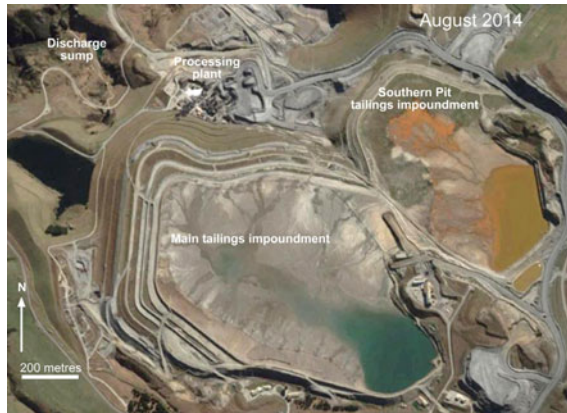
Fig. 10.6 Aerial view in 2014 of the two principal tailings impoundments at Macraes mine (from GoogleEarth). Brown waters in the impoundment to right result from autoclave discharge of iron oxyhydroxide, jarosite and ferric arsenate. A third impoundment (not shown) was also in use in 2014 (Chap. 1)
