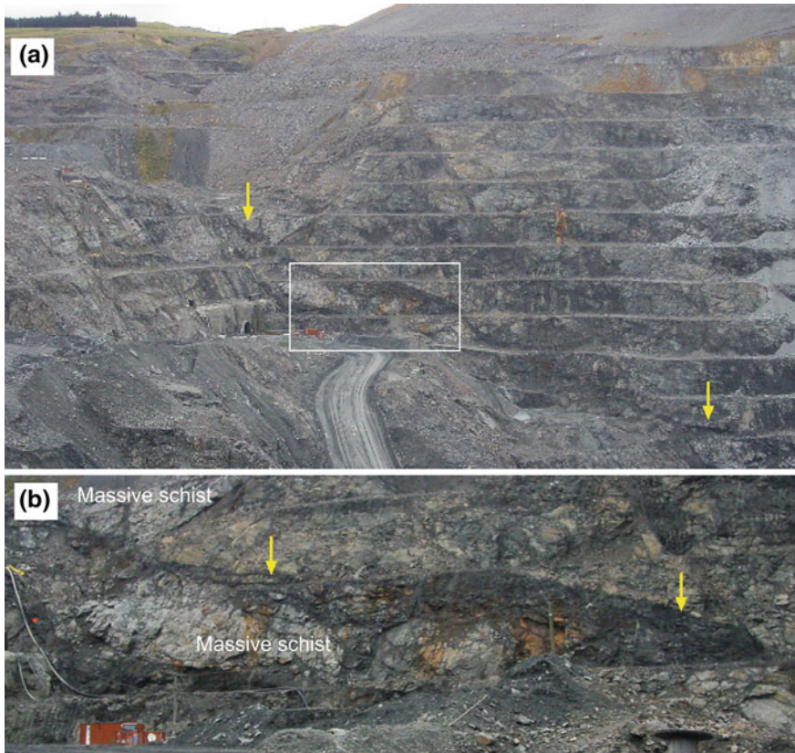
Fig. 3.8 The Hangingwall Shear (black sheared rocks, arrowed ) in the lower, most mineralised, part of the Hyde-Macraes Shear Zone in Frasers open pit. Other colour variations in the pit walls reflect lithological variations. a Shear dips down the northwest wall of the pit. Frasers underground mine portal is at centre left. b Closer view of the area indicated in (a) , with the Hangingwall Shear bending around pods of massive (mainly feldspathic) unmineralised schist
