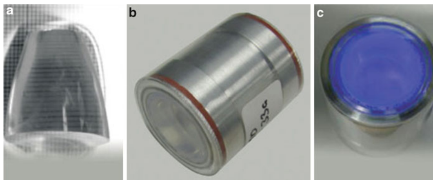
Fig. 22.1 (a) A crystal of strontium iodide doped with europium for gamma-ray detection is an R&D 100 Award winner. (b) The crystal is encapsulated when used in a radiation detection device and (c) glows blue when exposed to ultraviolet light
