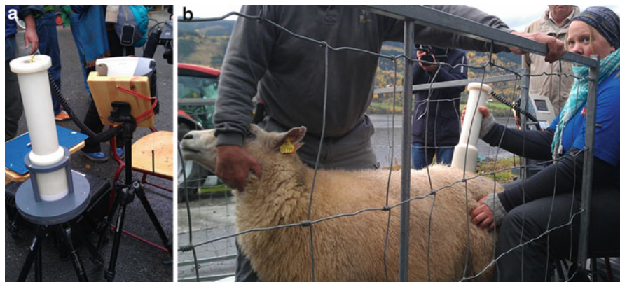
Fig. 19.2 (a, left): Equipment for live monitoring and (b, right): Position of the detector while measuring sheep (Photos: Astrid Liland, NRPA)
