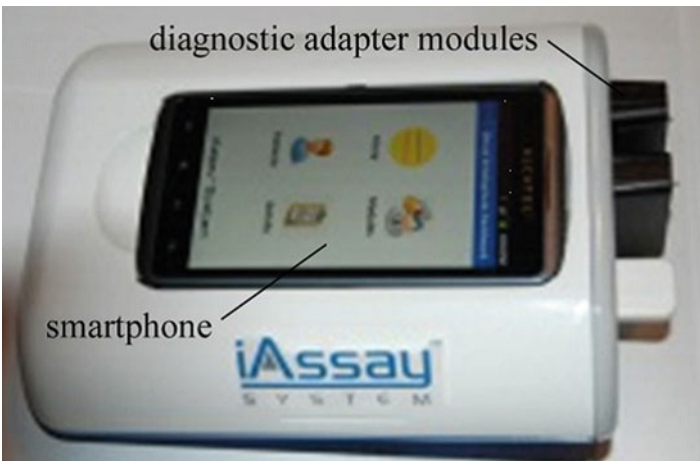
Fig. 22.4 iAssay ® diagnostic cartridge and smartphone interface
