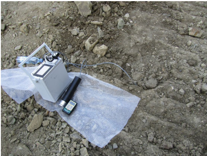
Fig. 9.7 A 2 M4000 monitor for measuring the Radon/Thoron soil gas activity and the local Gamma activity
