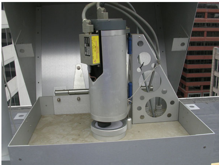
Fig. 11.4 RadNet fixed location monitor detectors
