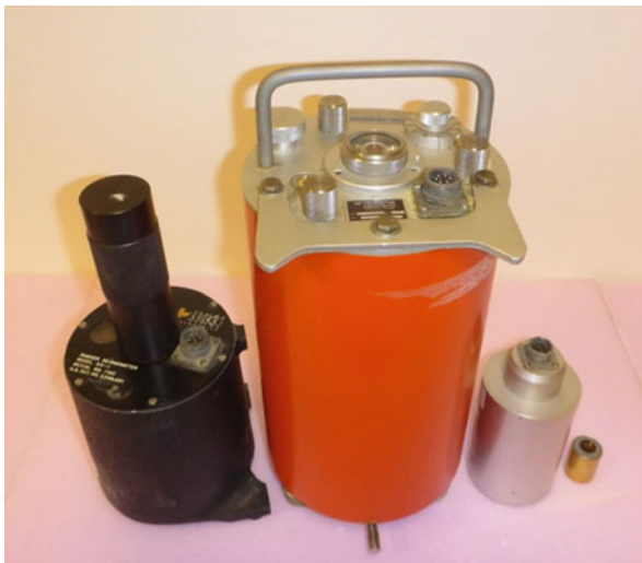
Fig. 2.53 Examples of passive sensors. From the left : (1) The Kinemetrics Ranger. Note the small window to the left for seeing the centering marks (screw under top cylinder), on the bottom there is a lock screw. (2) Teledyne S13: Note the small window in the center for observing the centering of the mass. The window can be unscrewed and there is access to place a weigh on the mass for calibration (see Chap. 10), there is a lock screw on the top. (3) The L4 sensor from Sercel. There is no centering or lock screw and the sensor should be transported upside down. (4) Typical 4.5 Hz geophone
