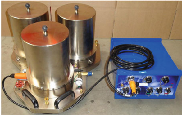
Fig. 2.56 Metrozet M2166-VBB Triaxial Seismometer System: Integrated triaxial sensor package (M2166-VBB-TSP) at left. M2166-EM Electronics Module at right. Each sensor axis is connected to electronics via dedicated cable. The electronics connect to a 3 or 6-channel Q330HR recorder via the connectors on the front side of its box. The weight is 68 kg and the power consumption is 5 W (Figure and some text from www.metrozet.com )
