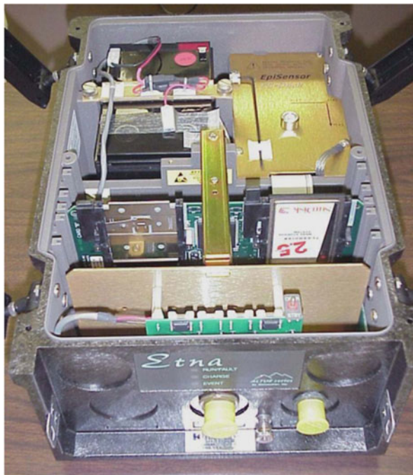
Fig. 5.18 The Kinematics Etna strong motion recorder, shown with the cover off. The battery is in the back (left) and the Episensor at the back right. The PCMCIA cards are seen in the middle. The size is 26 \times 38 \times 18 cm and the weight is 9 kg including the battery (From www.kinematics.com )
