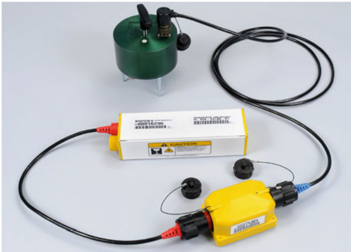
Fig. 5.14 The GeoSpace GSX recorder (box below) connected to a small battery and a GeoSpace three component geophone, MiniSeisMonitor, consisting of three HS-1 LT, 2.0 Hz geophones (see Table 2.3). The size is 7 \times 9 \times 12 cm (without connector) and weight is 0.9 kg (Figure from www.geospace.com )
