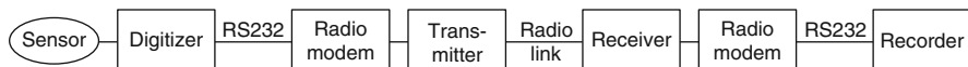
Fig. 8.15 One way communication from a remotely installed digitizer via a digital radio link to a centrally located PC. The radio modem and transmitter /receiver might be one unit
