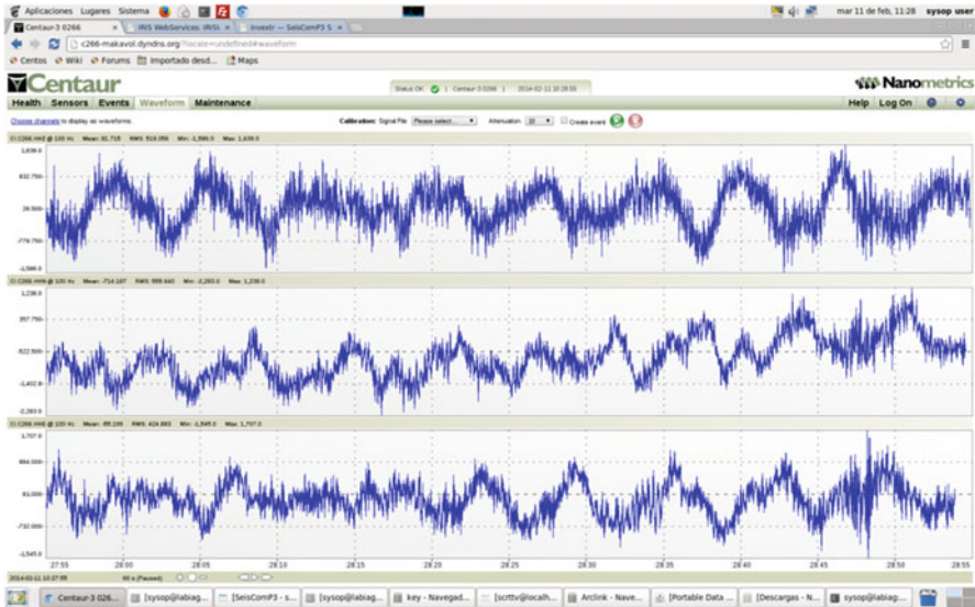
Fig. 8.21 Web interface of a Centaur recorder from Nanometrics. Any Web browser can be used to set the mode of operation, download events, etc. This snapshot shows the real time waveforms
