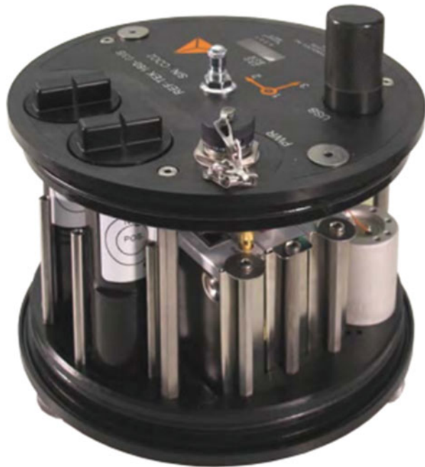
Fig. 5.24 The REFTEK 130S-01, a complete seismic station with two 3-channel internal sensors and a recorder. An SP sensor is seen to the right. The diameter is 22 cm and the height is 15 cm. the weight is 5.2 kg including battery and sensor
