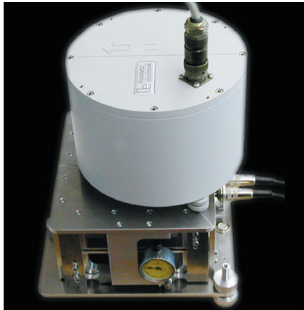
Fig. 10.15 An example of a calibration table. The table is moving vertically with no tilt. The vertical motion is measured by two mechanical gauges (accuracy 1 \mu\text{m} ) placed on each side (Figure from Lennartz-electronic.de)
