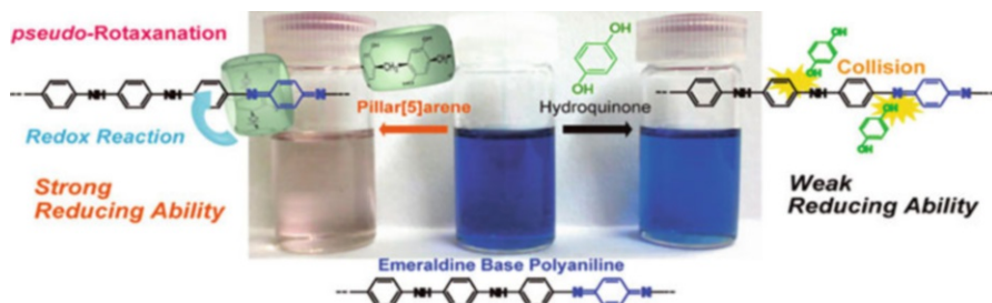
Fig. 2.8 Color change of the EB form of PANI upon addition of pillar[5]arene and hydroquinone and proposed structures in the reduction mechanism using hydroquinone and pillar[5]arene as reducing agents. (Reproduced with permission from Ref. [30]. Copyright 2011 American Chemical Society)
