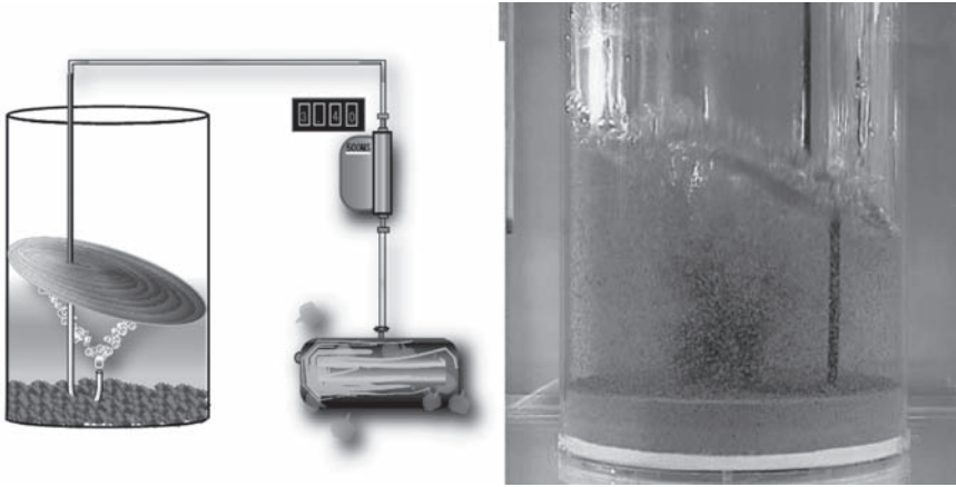
(a) Illustration of experimental device. (b) Photo showing particle flotation by bubbles.
