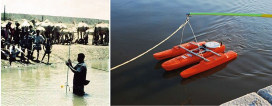
Fig. 3.3 Low flow gauging with a current meter ( left ) and an acoustic Doppler used to record measurements on Wild Rice River, North Dakota, during 2010 flood ( right , US Geological Survey/ photo by Don Becker http://gallery.usgs.gov/ )
