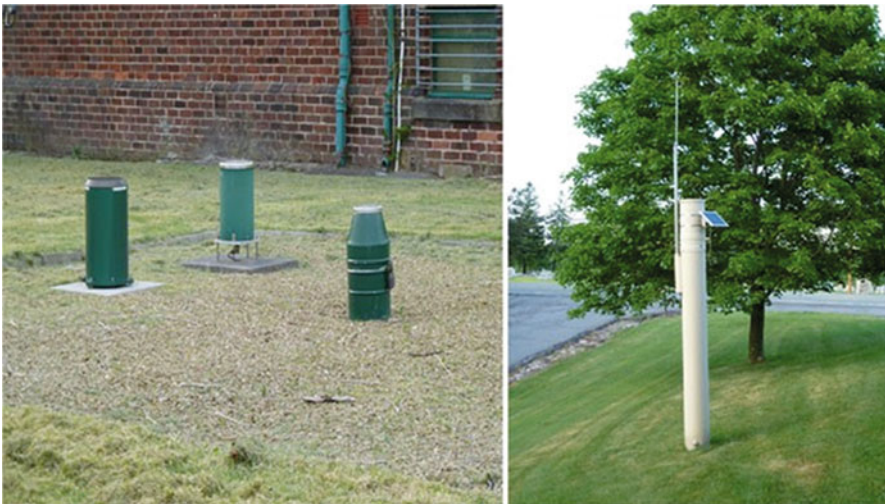
Fig. 2.3 Examples of raingauges sited at a weather station in the UK ( left ) and an IFLOWS installation in the USA ( right ). Integrated Flood Observing and Warning Systems (IFLOWs) are widely used in flood warning applications in the eastern USA and have similar origins to the ALERT systems discussed in Chap. 3; here, the gauge is situated at the top of the structure, which also houses a data logger and telemetry equipment (Sene 2013)
