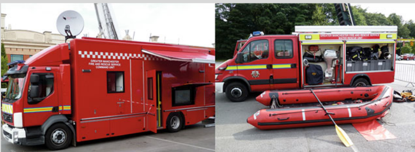
Fig. 7.5 Command Unit and Water Rescue Unit used by the Greater Manchester Fire and Rescue Service in the UK during flood and other emergencies. The computer screen on the side of the command unit is used for briefing staff and shows the locations of key vehicles and other assets against a map-based background; there are additional displays in the vehicle together with computer workstations and communications equipment
