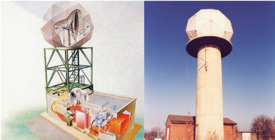
Fig. 2.6 View of the internal workings of a weather radar and the Chénies Radar in the UK (Met Office 2013; Contains public sector information licensed under the Open Government Licence v1.0)
