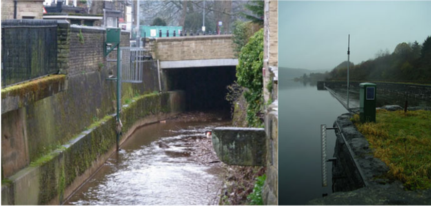
Fig. 3.1 Examples of pressure transducer installations in an urban river and in a reservoir (with associated gauge boards)
