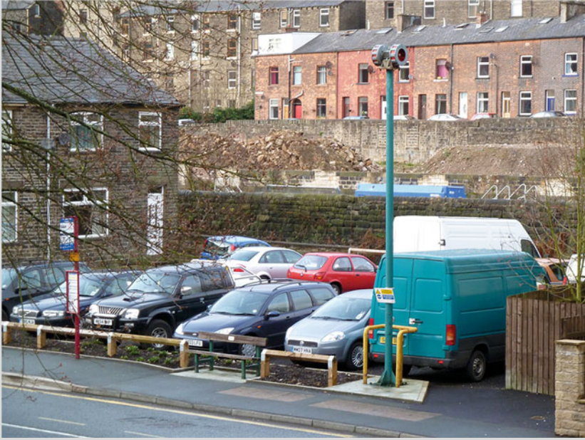
Fig. 7.2 Example of a flood warning siren in Northeast England: the river lies between the two flood walls behind the siren (Adapted from Sene 2013)
