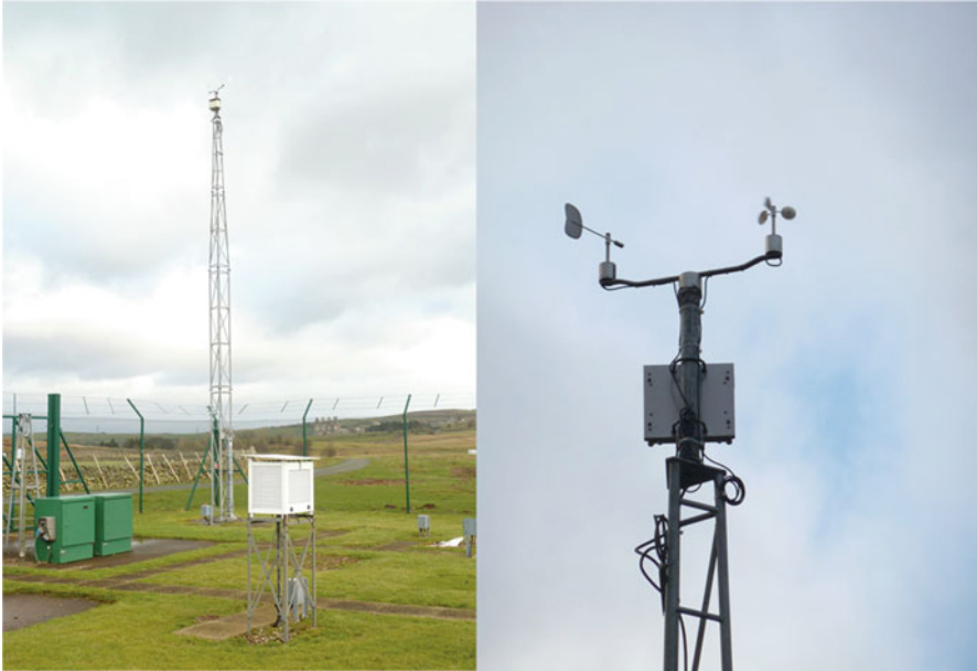
Fig. 2.4 Example of a weather station in the UK with a Stevenson Screen in the foreground and a mast with a cup anemometer and wind vane; the inset image shows the top of the mast in more detail
