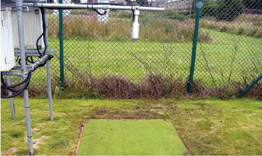
Fig. 3.6 Snow depth sensor (Met Office 2010; contains public sector information licenced under the Open Government Licence v1.0)
