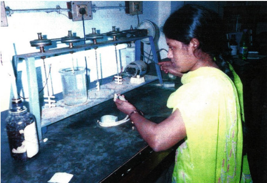
Exhibit 12.6 Setting flash mixing speed with several RPM
