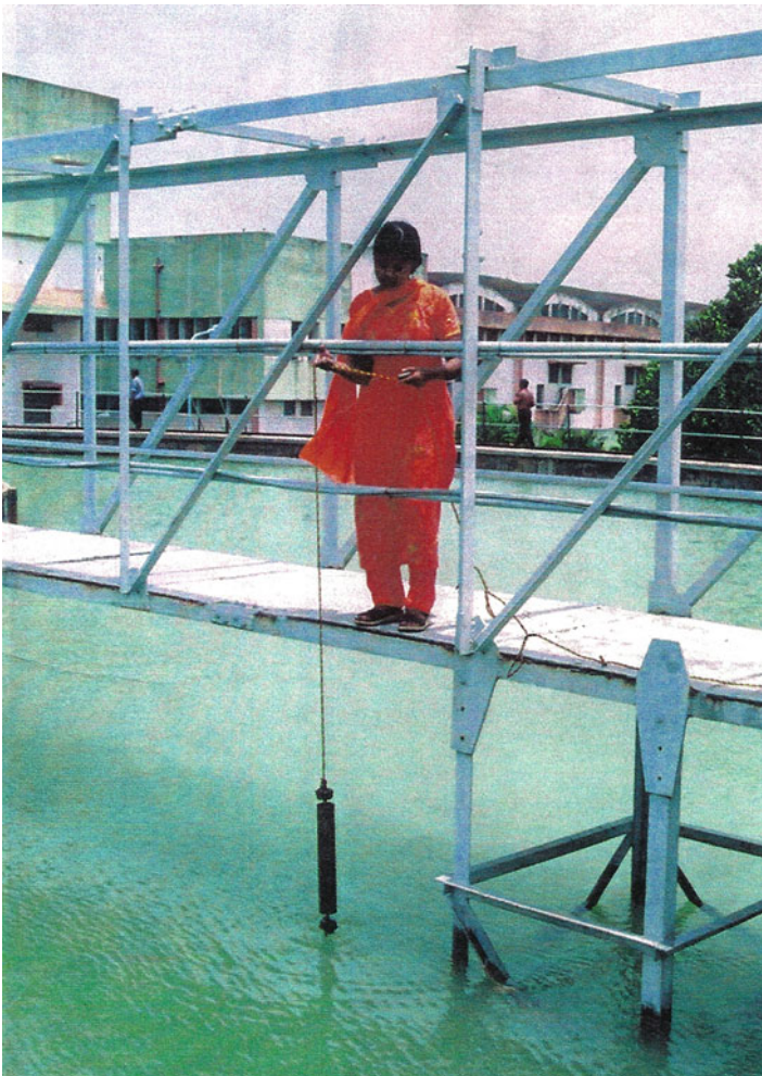
Exhibit 12.7 Depth-wise sampling using Kemmerer sampler
