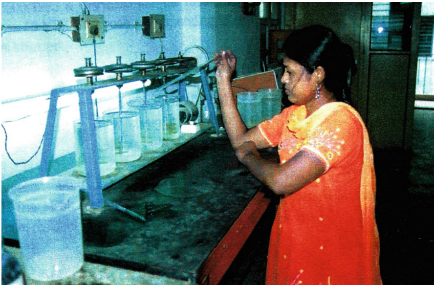
Exhibit 12.4 Jar test to determine coagulant dosage
