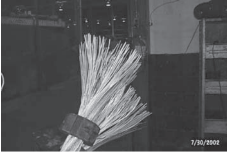
Figure 1. Individual wires in broom configuration.
