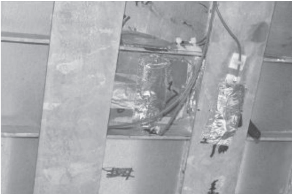
Figure 7. Strain gauge placement.
