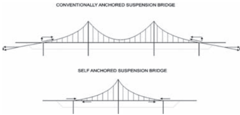
Figure 7. Suspension bridges (Fukuhara, 2005).
