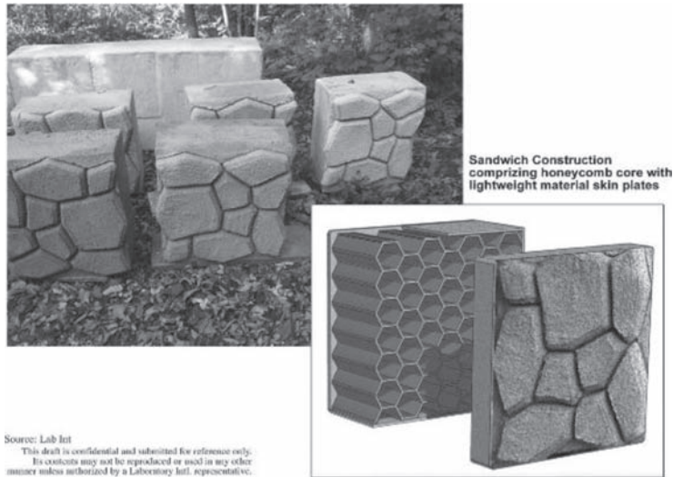
Figure 1. Caption of sample Lightweight material blocks and an illustration of “Sandwich Construction” for ultra lightweight support application.
