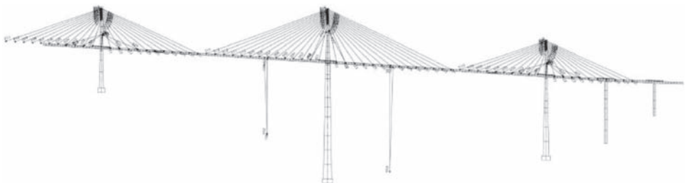
Figure 4. Structural model for the assessment of the residual bearing capacity of Mezcala Bridge (Mexico) after 2007 major road accident.
