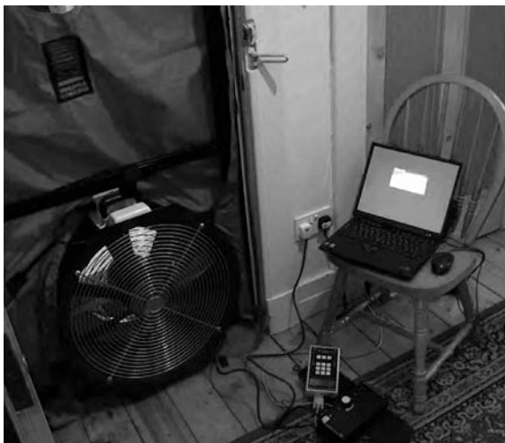
Fig. 1 Air-tightness testing in a tenement flat [21]
