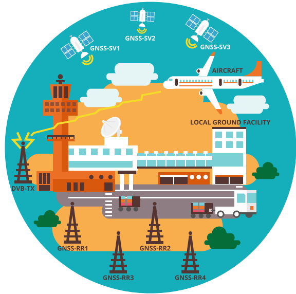
Fig. 5.1 Main component of a local-area augmentation system
