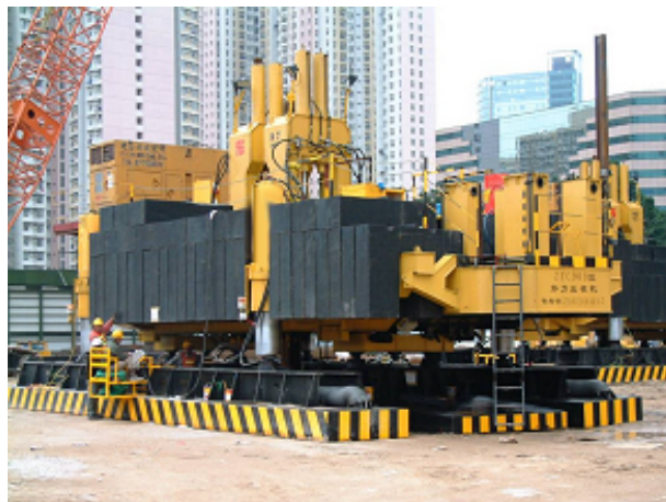
Plate 4.3 – A Pile Jacking Machine
