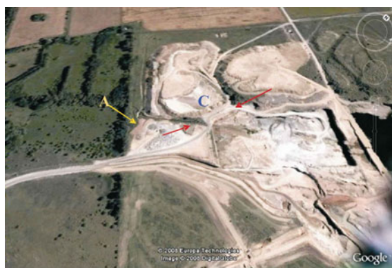
Fig. 5.6 View of the opening of the La Pampita quarry, Loma Negra, Sierras Bayas. Arrows indicate the north–south front, where the study was carried out. A Clays of the Olavarría Formation. C Limestones of the Loma Negra Formation. The image was captured using the publicly available software Google Earth ( http://earth.google.com/ ). Copyright 2008 DigitalGlobe; Europa Technologies
