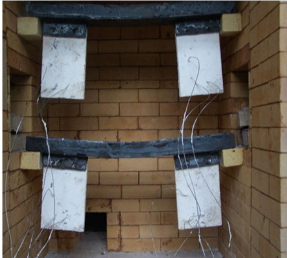
Fig. 4.5 Small-scale samples hinged in furnace
