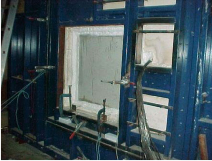
Fig. 4.8 A exterior view of the furnace used in test on steel members [18]
