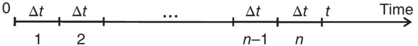
Figure 3.10 A time interval (0, t) divided into n small intervals with lengths \Delta t
