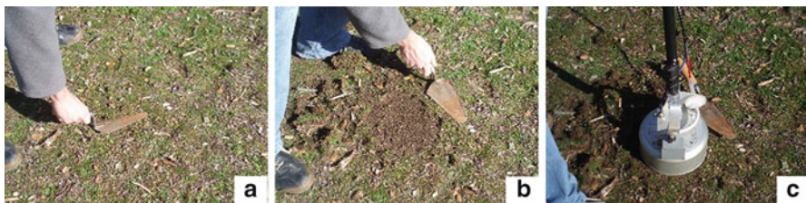
Fig. 2 Protocol of \text{CO}_2 measurement (a). Cleaning, (b). Waiting and (c). Measuring
