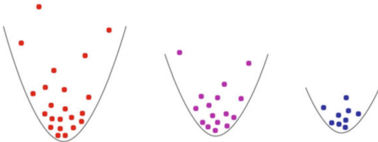
Fig. 1 Cooling of atoms by evaporation in a magnetic trap
