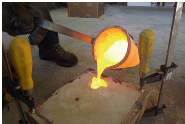
Fig. 4.3 Bronze founding; the “mouth” or “breathing hole” is clearly visible. Photograph by Steve Hoerner
