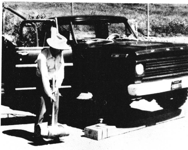
FIGURE 49. Horizontal traction or plate and hammer method used for identifying subsurface layers of rock or soil plus their configurations and elastic properties. Mechanics of the method are described in the text. (Courtesy of Jay H. Power, California Division of Mines and Geology.)
