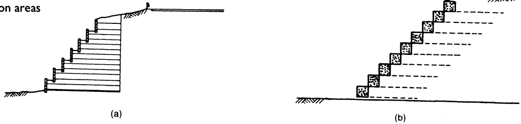
Fig. 3.22. (a) Stepped embankment or retaining wall; (b) gabion faced reinforced soil structure
