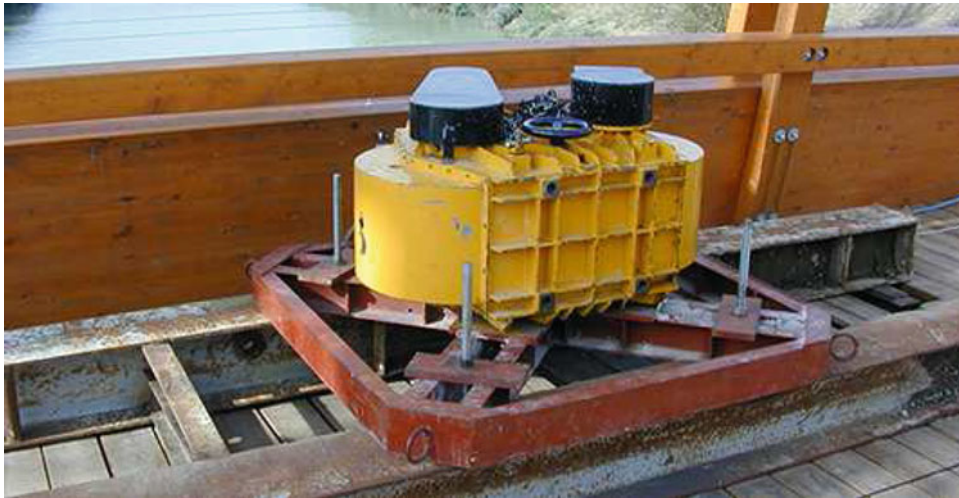
Fig. 26.2 Mechanical shaker in position 1 (horizontal forces)
