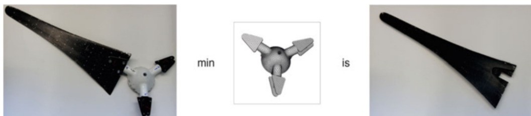
Fig. 10.3 Schematic of the one blade substructuring problem
