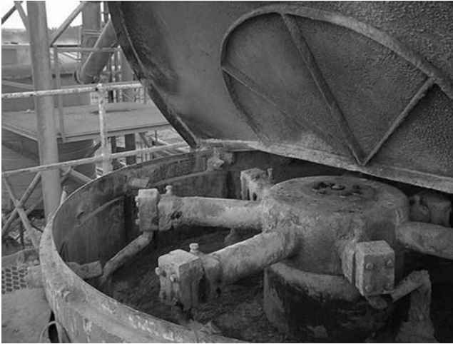
Figure 10.2 Inside of modern mobile pan mixer.
