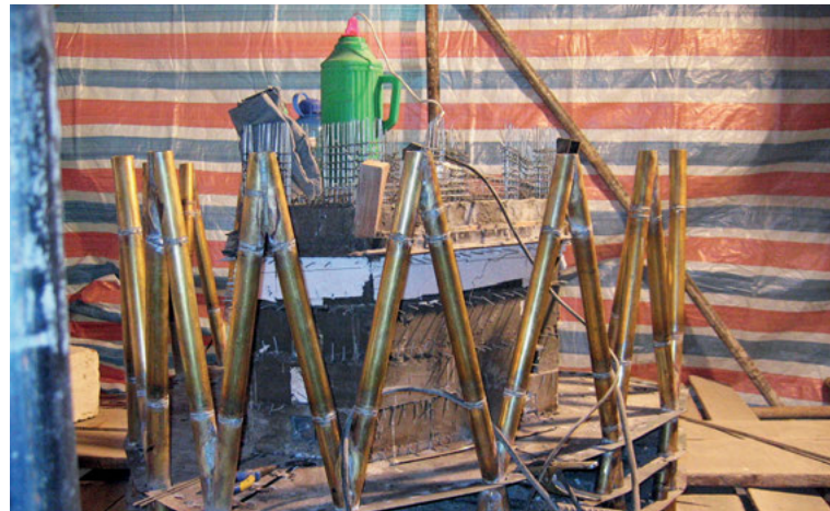
A large-scale model of the Guangzhou IFC in Guangzhou, China, designed by Wilkinson Eyre Architects with Arup. The innovative nature of the application of these large diagrid structures necessitates methods of exploration and structural validation that often include the construction of large physical models.
