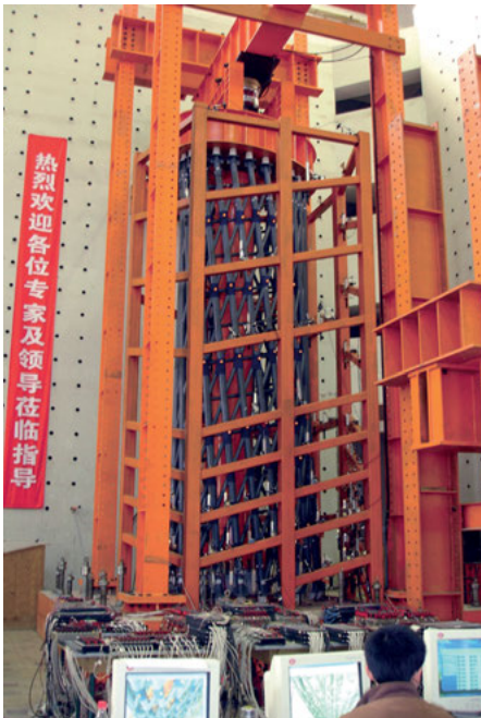
A large-scale model of the Guangzhou IFC in Guangzhou, China, designed by Wilkinson Eyre Architects with Arup. The innovative nature of the application of these large diagrid structures necessitates methods of exploration and structural validation that often include the construction of large physical models.
