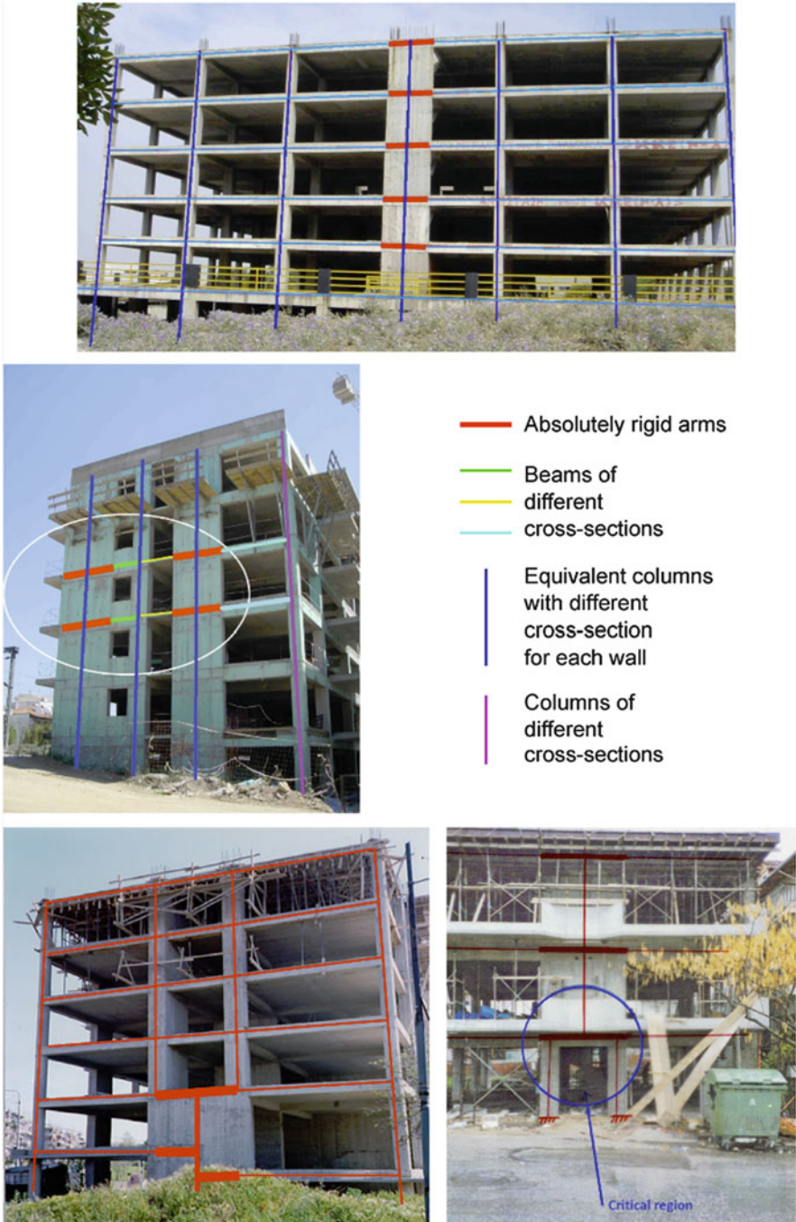
Fig. 2.41 Equivalent frame models for structural walls in r/c building (Rigid joints in column-beam connections are omitted)
