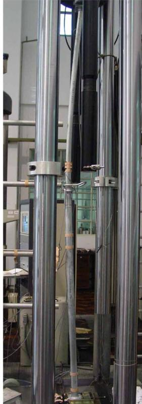
Figure 40. Behaviour under axial loading of an imperfect steel telescopic prop
