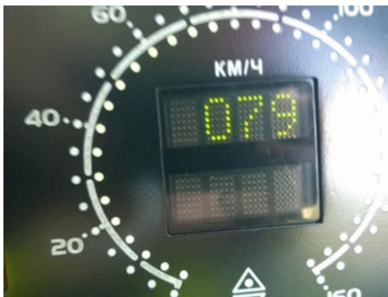
Fig. 66 Driver’s display data during braking system tests of the platform MPP-61 No. 00000001 at a speed of 80 km/h
