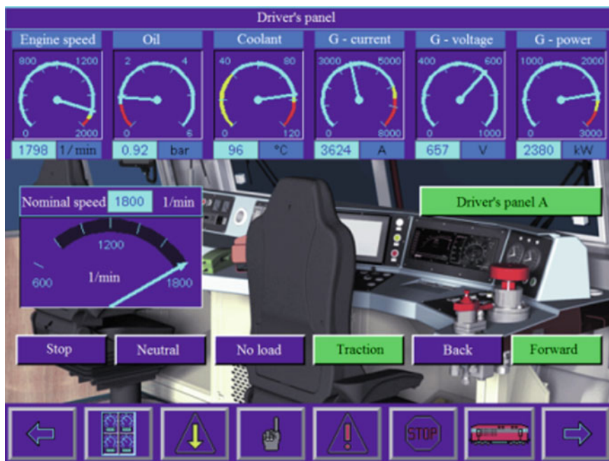
Fig. 43 Information window in the diagnostics display of control panel A in the diesel-electric locomotive TEP-70
