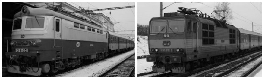
Fig. 2 Locomotive type 242 with a diode rectifier, ( DPF \cong 0.84 ) and locomotive type 263 with a thyristor-diode bridge, ( DPF \cong 0.77 )
