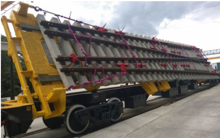
Fig. 68 Photo of platform MPP-61 with three-component tilted cargo lifting equipment with cargo
