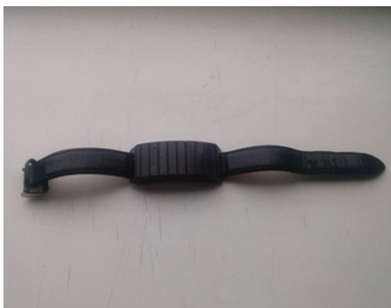
Fig. 43 Driver's alertness checking bracelet
