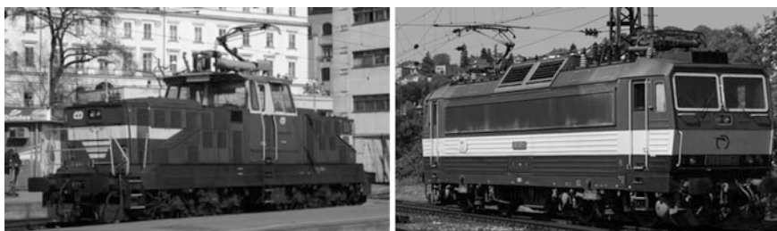
Fig. 3 Locomotive type 210 with a thyristor controller and uncontrolled rectifier, ( DPF \cong 0.76 ) and locomotive type 362 with an input converter filter, ( DPF \cong 0.87 )
