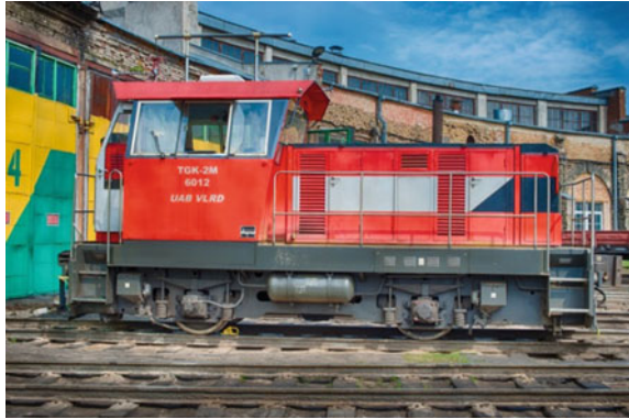
Fig. 77 Shunting locomotive TGK-2
