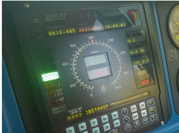
Fig. 64 Driver’s display data during braking system tests of the platform MPP-61 No. 00000001 at a speed of 60 km/h
