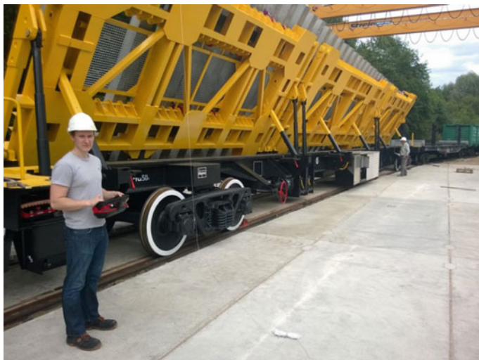
Fig. 70 Photo of the functional performance testing of lifting-lowering of platform MPP-61 No. 00000001 with fixed cargo
