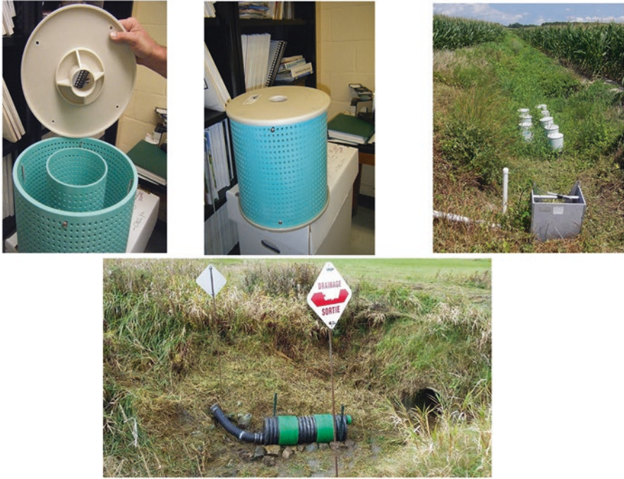
Fig. 3.11 Examples of a cartridge style P removal structure. For the three upper photos, the principal is the same as the modular box shown in Fig. 3.8 The outer-ring is filled with PSM and water flows through the PSM into the center ring, which is connected to a pipe at the bottom for transferring the treated water. The photo on the upper right shows several cartridges installed in a drainage ditch with a flow-control structure for maintaining hydraulic head. Lower photograph shows a cartridge style P removal structure that treats a subsurface tile drain. While designed for easy cleanout/replacement, the small mass of PSM contained is a major disadvantage. Upper photo credits: Gene Hahn, University of Kentucky. Lower photo is courtesy of Barry Husk, Blue Leaf Inc.
