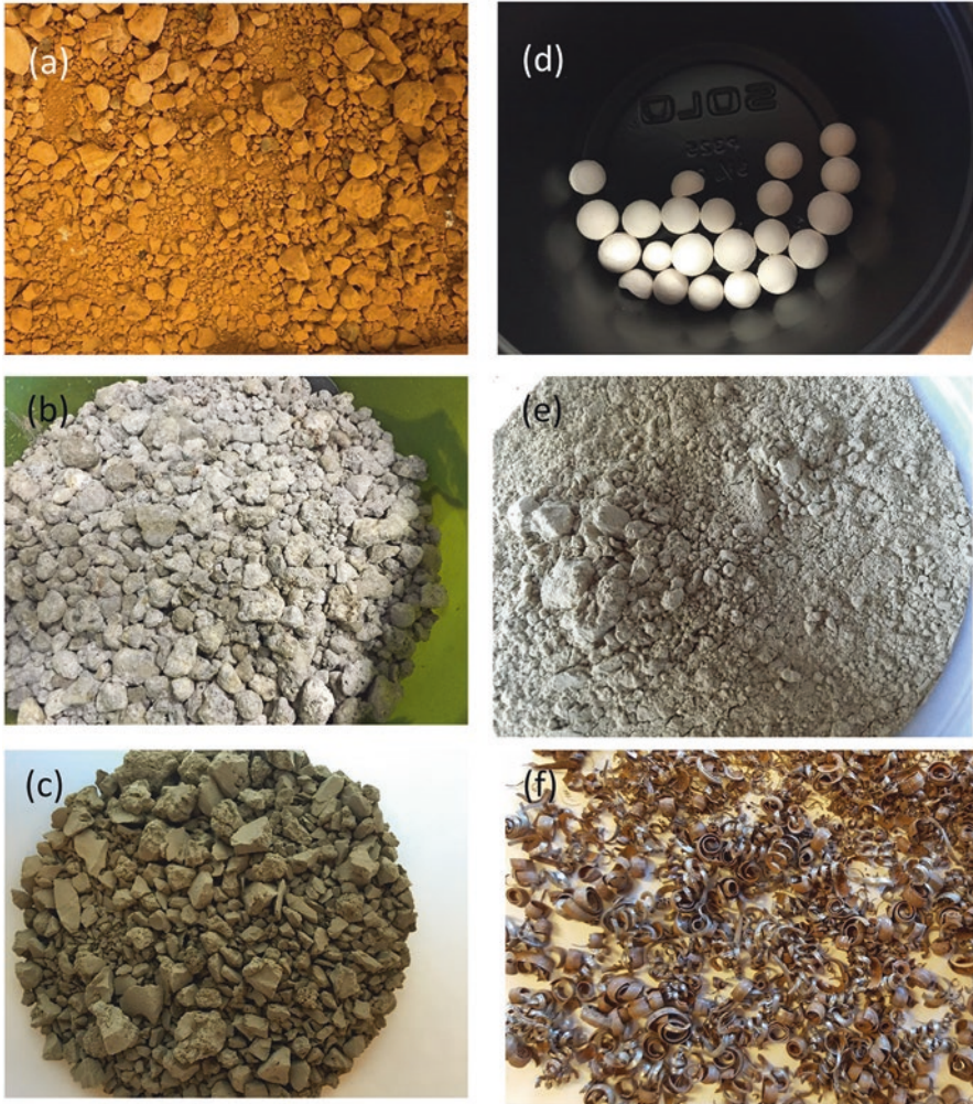
Fig. 4.1 Examples of several potential PSMs: (a) acid mine drainage residuals (AMDRs), (b) steel slag, (c) drinking water treatment residuals (WTRs), (d) manufactured PSM known as “Blue Leaf”, (e) fly-ash, and (f) metal shavings. Photo credit: James Bowen and Joshua Bradley
