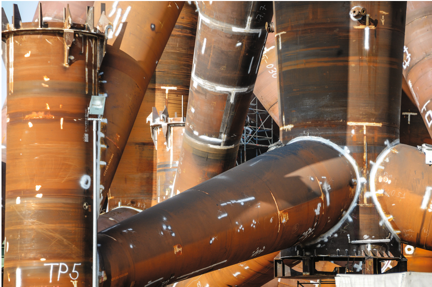
Fig. 1.2 Support structures: thick-walled welded steel constructions
