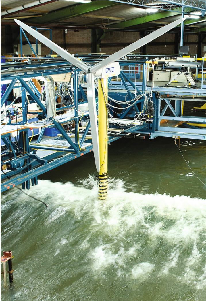
Fig. 8.1 Breaking waves contribute significantly to the mechanical loading of an offshore wind turbine structure
