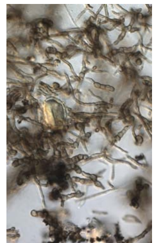
Figure 4.1-E Mold Growth (Spores and Hyphae) on the Dust and Dirt on a Metallic Airstream Surface Photograph courtesy of Phil Morey.
