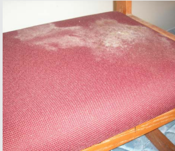
Figure 2.3-B Mold Growth due to Negative Pressure
