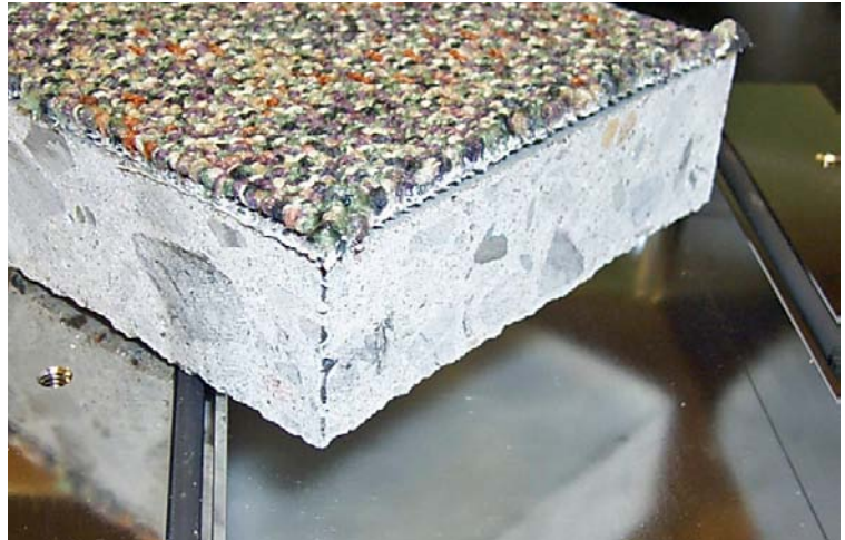
Figure 5.1-I Carpet/Adhesive/Concrete Test Assembly Photograph copyright NRC.
