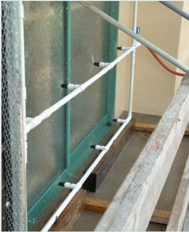
Figure 1.2-I Water Spray Test Assembly in Use Photograph courtesy of Dave MacPhaul; copyright CH2M HILL.
