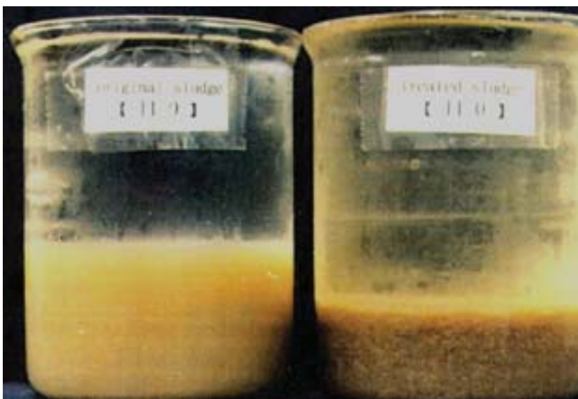
Fig. 1. The appearance of the collected activated sludge sample collected from a food manufacturing plant.
