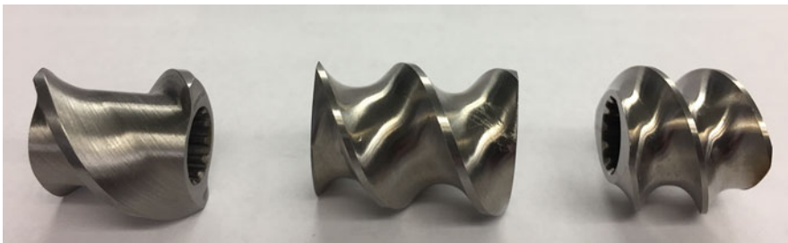
Fig. 6.15 Example conveying screws (from left to right: 2 S/D, 1.5 S/D, and 1 S/D)
