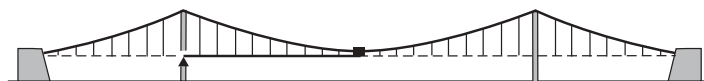
Figure 3.48 Three-span suspension bridge with a central clamp and a fixed bearing at one of the pylons
