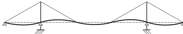
Figure 3.204 Stiffening girder oscillating independently of the cable system in a bridge with only one set of stays from each pylon
