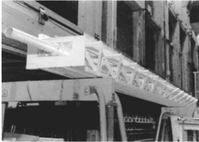
Figure 8.15 Sectional model of the Øresund Bridge before erection in the wind tunnel
