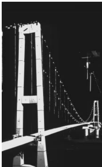
Figure 8.14 Full model of the Storebælt Bridge in the large 13.6 m wide wind tunnel at Danish Maritime Institute, Denmark
