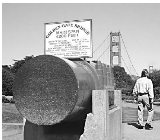
Figure 2.21 Mock-up of the Golden Gate Bridge main cable composed of 27 572 wires
