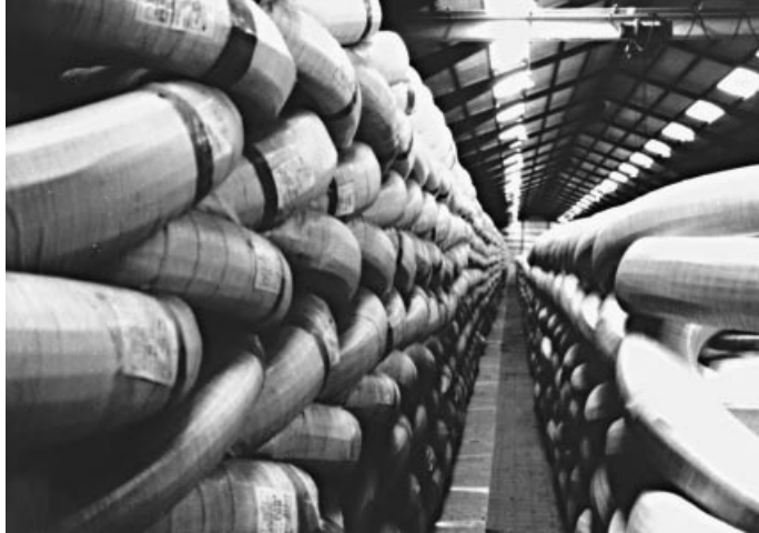
Figure 2.88 Wire reels for the Storebælt East Bridge
