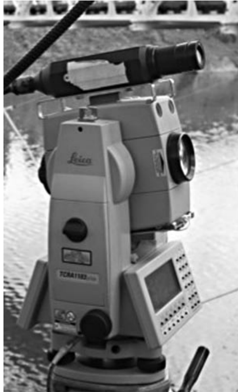
Figure 9.19 Total station (TPS) with high power Laser Doppler Velocimeter (Photo credit: Y. Fujino)
