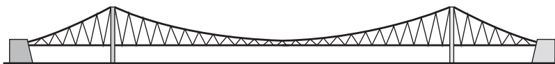
Figure 3.57 Suspension system with inclined hangers between the main cable and the deck
