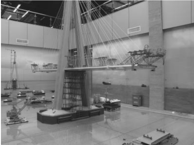
Figure 7.68 Model of the Sutong Bridge during free-cantilever erection of the deck
