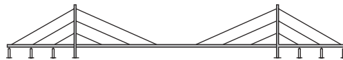
Figure 3.118 Structural system of a bridge with harp systems and intermediate supports in the side spans
