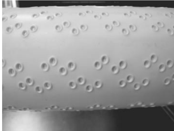
Figure 8.41 Pattern-indentated HDPE tubing used on Sutong and Stonecutters Bridges
