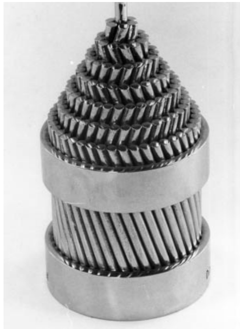
Figure 2.2 Multi-wire helical strand (Lillebælt Bridge)
