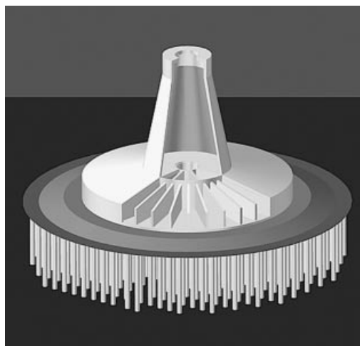
Figure 9.15 Rion-Antirion Bridge foundation
