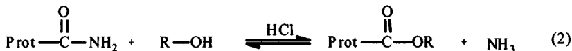
Figure 1. Esterification of carboxylic acid (1) and amide groups (2) of proteins by an aliphatic alcohol
