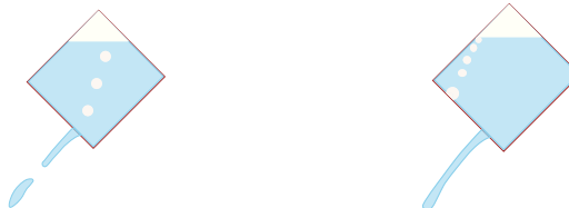
Fig. -8.11. Counter-current flow in a can (the left figure) has only one hole thus pulse flow and a flow with two holes (right picture).
