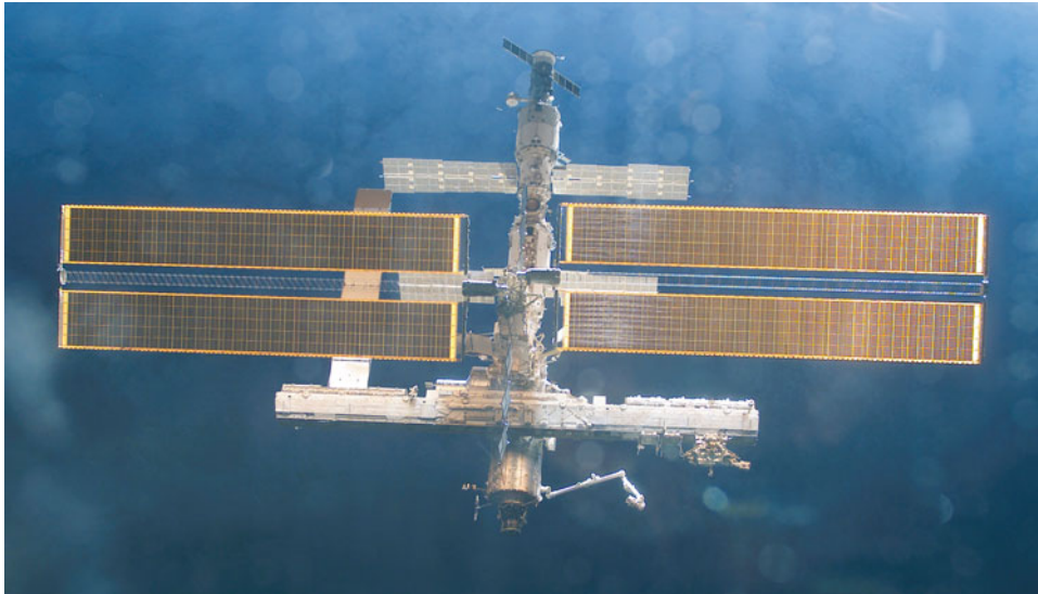
The ISS with the P1 and S1 truss segments in place. Note the presence of the MBS and both CETA carts on the S1 truss (on the right side of this view). (NASA)
