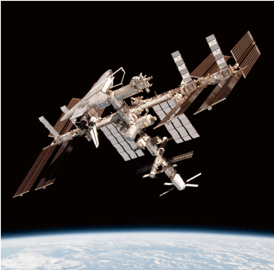
The ISS with Endeavour and the ATV-2 ‘Johannes Kepler’ docked at opposite ends of the station. This photograph was taken by Paolo Nespoli aboard Soyuz TMA-20. (ESA)
