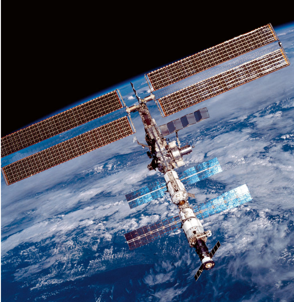
The configuration of the ISS during STS-105 (previous mission) showing Destiny and the Quest Joint Airlock. (NASA)
