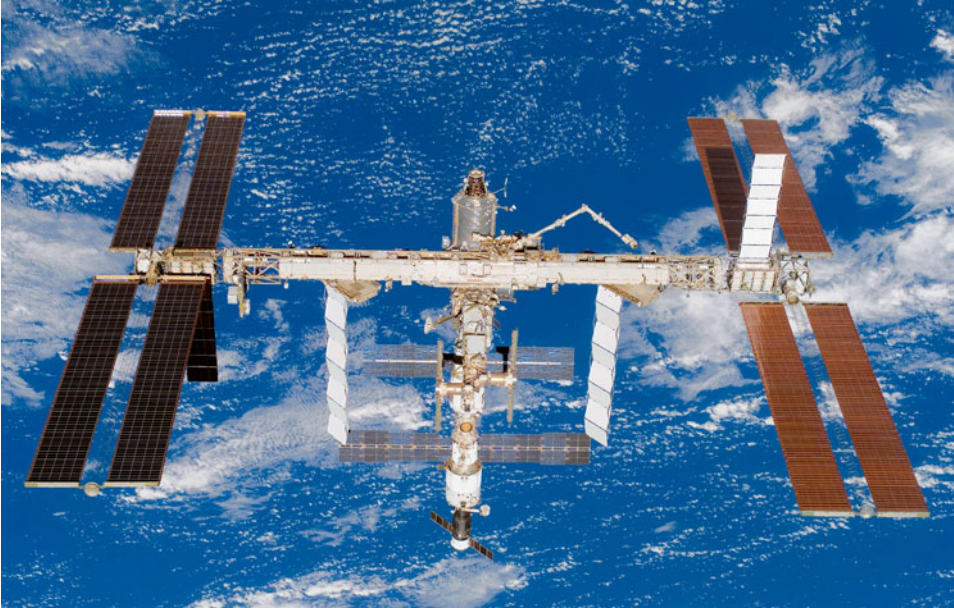
The ISS after the STS-118 mission, showing the S3/S4 truss segments and solar arrays delivered by STS-117 matching the P3/P4 truss segments delivered by STS-115. (NASA)
