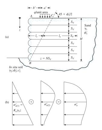
Figure 13.27 Analysis of a reinforced-earth retaining wall
