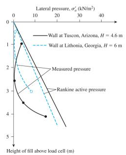
Figure 13.38 Comparison of theoretical and measured lateral pressures in geogrid reinforced retaining walls (Based on Berg et al., 1986)
