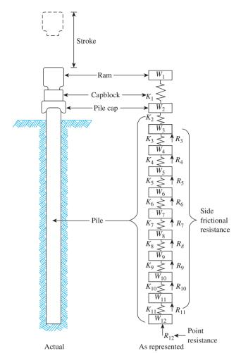
**Figure 9.39** Wave equation model for driven piles (Based on Smith, 1960)
