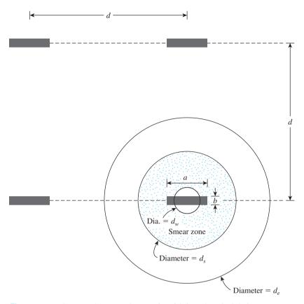
Figure 16.27 Square-grid pattern layout of prefabricated vertical drains
