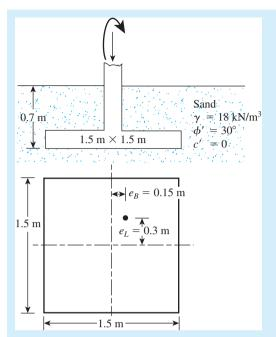
Figure 4.30 An eccentrically loaded foundation
