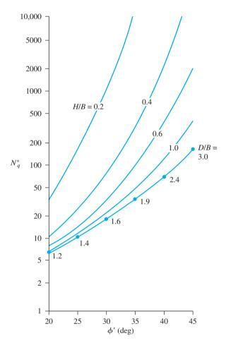
Figure 5.4 Mandel and Salencon's bearing capacity factor  $N_q^*$  [Eq. (5.2)]
