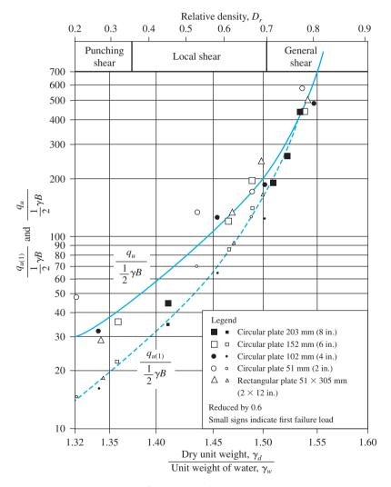
**Figure 4.2** Variation of  $q_{u(1)}/0.5\gamma B$  and  $q_u/0.5\gamma B$  for circular and rectangular plates on the surface of a sand (Adapted from Vesic, 1963) (Based on Vesic, A. B. Bearing Capacity of Deep Foundations in Sand. In Highway Research Record 39, Highway Research Board, National Research Council, Washington, D.C., 1963, Figure 28, p. 137.)
