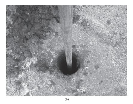
Figure 3.20 Sampling with a thin-walled tube: (a) tube being attached to drill rod; (b) tube sampler pushed into soil (Courtesy of Khaled Sobhan, Florida Atlantic University, Boca Raton, Florida)
