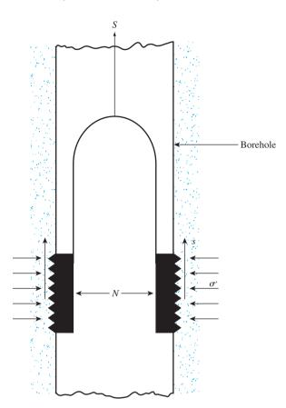
Figure 3.37 Iowa borehole shear test
