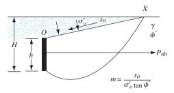
Figure 14.41 Assumed failure surface in soil for stress characteristic solution
