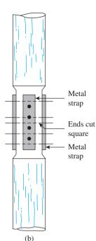
Figure 9.5 Splicing of timber piles: (a) use of pipe sleeves; (b) use of metal straps and bolts
