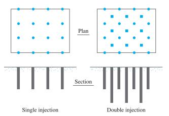
**Figure 11.22** Multiple lime slurry injection planning for a building pad
