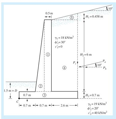
Figure 13.12 Calculation of stability of a retaining wall
