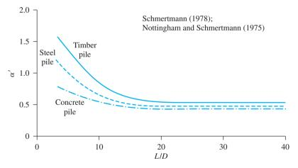
**Figure 9.19** Variation of  $\alpha'$  with embedment ratio for piles in sand: mechanical cone penetrometer
