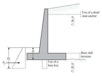
Figure 13.9 Alternatives for increasing the factor of safety with respect to sliding
