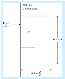
Figure 8.19 Critical perimeter column
