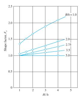
Figure 14.43 Variation of shape factor with H/h and B/h (Based on Neeley et al., 1973.)
