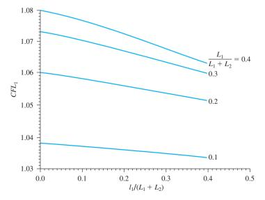
Figure 14.23 Variation of  $CFL_1$  with  $L_1/(L_1 + L_2)$  and  $l_1/(L_1 + L_2)$  [Based on Hagerty, D. J., and Nofal, M. M. (1992). "Design Aids: Anchored Bulkheads in Sand," Canadian Geotechnical Journal, Vol. 29, No. 5, pp. 789–795.]
