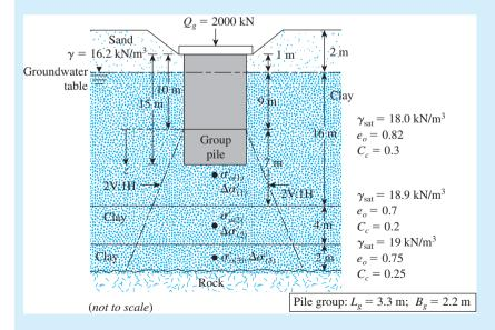
Figure 9.51 Consolidation settlement of a pile group
