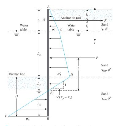
Figure 14.18 Anchored sheet-pile wall penetrating sand
