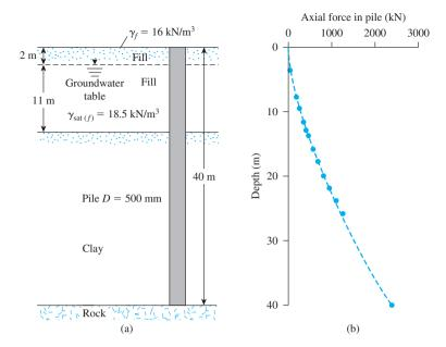
Figure 9.43 Negative skin friction on a pile in the harbor of Oslo, Norway (Based on Bjerrum et al., (1969) and Wong and The (1995))
