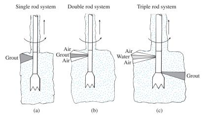
Figure 16.41 Jet grouting
