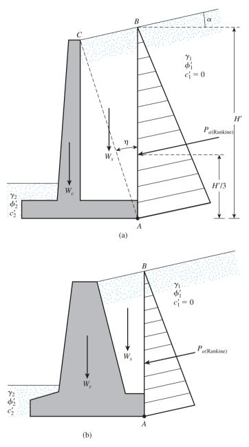
Figure 13.4 Assumption for the determination of lateral earth pressure: (a) cantilever wall; (b) and (c) gravity wall
