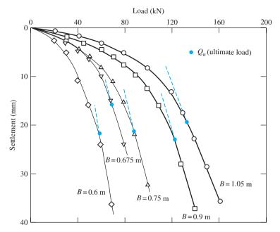
Figure 4.15 Load-settlement plots obtained from bearing capacity tests
