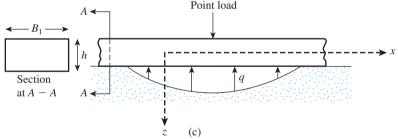
Figure 8.11 (a) Principles of design by conventional rigid method; (b) principles of approximate flexible method; (c) derivation of Eq. (8.42) for beams on elastic foundation
