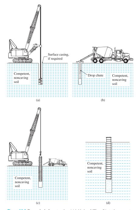
Figure 10.2 Dry method of construction: (a) initiating drilling; (b) starting concrete pour; (c) placing rebar cage; (d) completed shaft (Based on O'Neill and Reese, 1999)
