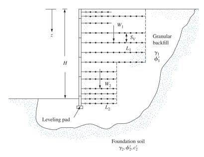
Figure 13.39 Design of geogrid-reinforced retaining wall
