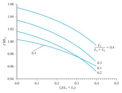
**Figure 14.24** Variation of  $CML_1$  with  $L_1/(L_1 + L_2)$  and  $l_1/(L_1 + L_2)$  [Based on Hagerty, D. J., and Nofal, M. M. (1992). "Design Aids: Anchored Bulkheads in Sand," Canadian Geotechnical Journal, Vol. 29, No. 5, pp. 789–795.]
