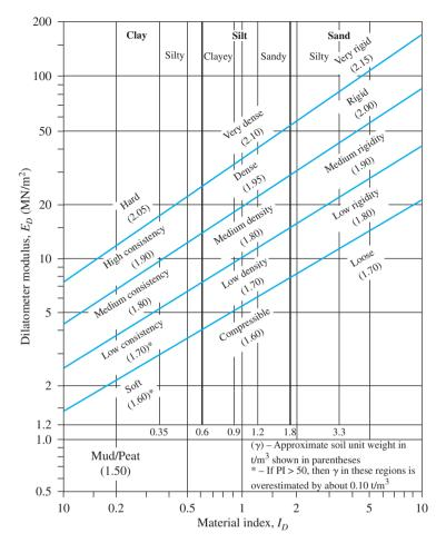
Figure 3.36 Chart for determination of soil description and unit weight (After Schmertmann, 1986) (*Note*:  $1 \text{ t/m}^3 = 9.81 \text{ kN/m}^3$ ) (Based on Schmertmann, J.H. (1986). "Suggested method for performing that flat dilatometer test," Geotechnical Testing Journal, ASTM, Vol. 9, No. 2, pp. 93-101, Fig. 2.)
