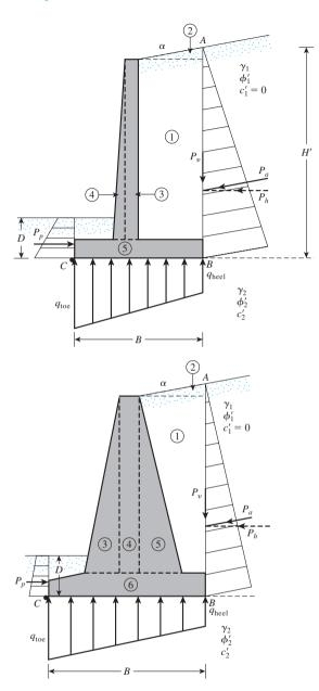
**Figure 13.7** Check for overturning, assuming that the Rankine pressure is valid
