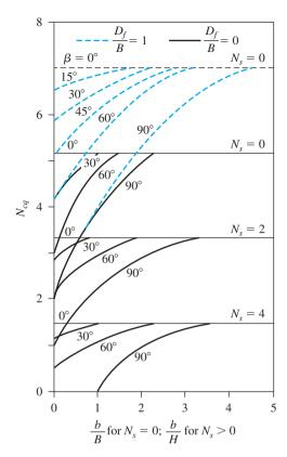
Figure 5.21 Meyerhof's bearing capacity factor  $N_{cq}$  for purely cohesive soil
