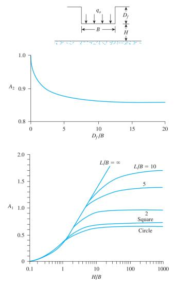
Figure 7.1 Values of  $A_1$  and  $A_2$  for elastic settlement calculation—Eq. (7.1) (After Christian and Carrier, 1978) (Based on Christian, J. T. and Carrier, W. D. (1978). "Janbu, Bjerrum and Kjaernsli's chart reinterpreted," *Canadian Geotechnical Journal*, Vol. 15, pp. 123–128.)
