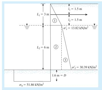
Figure 14.34 Free earth support method, with sheet pile penetrating into clay
