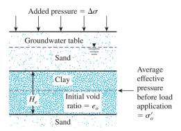
Figure 2.19 One-dimensional settlement calculation
