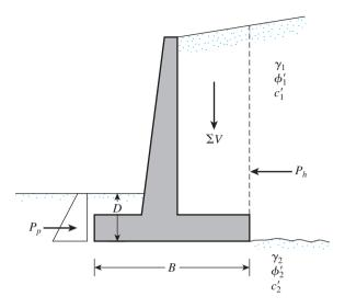
Figure 13.8 Check for sliding along the base
