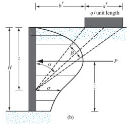
Figure 12.14 Lateral earth pressure caused by (a) line load and (b) strip load
