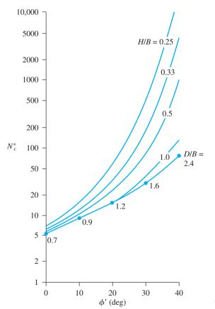
Figure 5.3 Mandel and Salencon's bearing capacity factor  $N_c^*$  [Eq. (5.2)]
