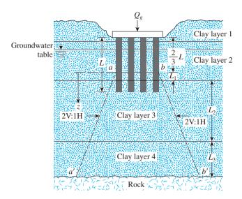
Figure 9.50 Consolidation settlement of group piles
