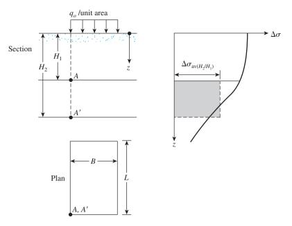
**Figure 6.12** Average pressure increase between  $z = H_1$  and  $z = H_2$  below the corner of a uniformly loaded rectangular area
