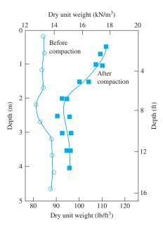
Figure 11.7 Dynamic compaction of a friable loess layer in Russe, Bulgaria (Based on Lutenegger, 1986)
