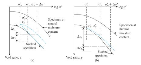
Figure 11.4 Settlement calculation from double oedometer test: (a) normally consolidated soil; (b) overconsolidated soil
