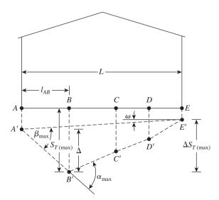
Figure 7.27 Definition of parameters for differential settlement
