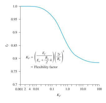
Figure 7.7 Variation of rigidity correction factor  $I_F$ with flexibility factor  $K_F$ [Eq. (7.18)]
