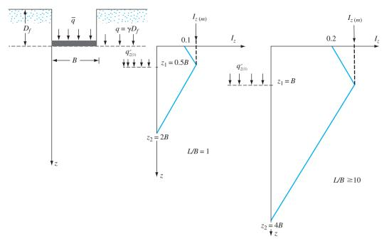
**Figure 7.9** Variation of strain influence factor with depth and L/B
