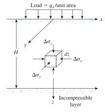
Figure 7.2 Elastic settlement of shallow foundation
