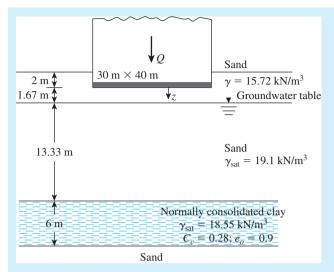
**Figure 8.9** Consolidation settlement under a mat foundation
