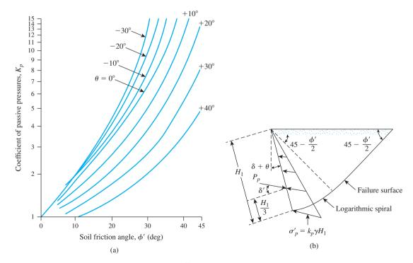
**Figure 12.23** Caquot and Kerisel's solution for  $K_p$  [Eq.(12.68)]
