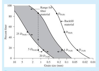
Figure 13.16 Determination of grain-size distribution of filter material
