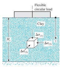
Figure 7.21 Circular foundation on a clay layer
