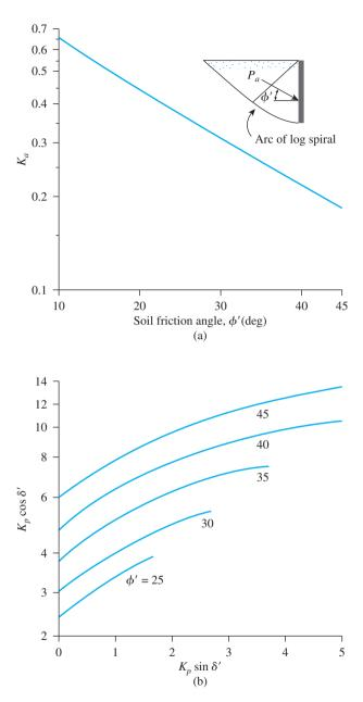
**Figure 14.38** (a) Variation of  $K_a$  for  $\delta' = \phi'$ , (b) variation of  $K_p \cos \delta'$ with  $K_p \sin \delta'$  (Based on Ovesen and Stromann, 1972)
