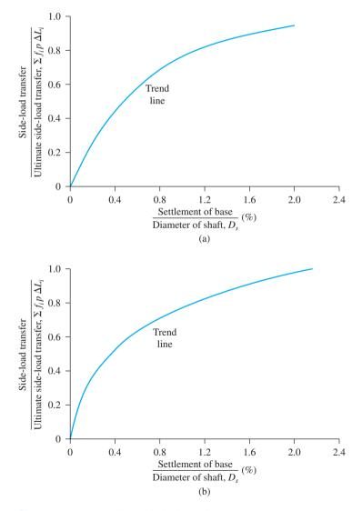
Figure 10.13 Normalized side-load transfer versus settlement: (a) gravelly sand (gravel 25 to 50%) and (b) gravel (more than 50%)
