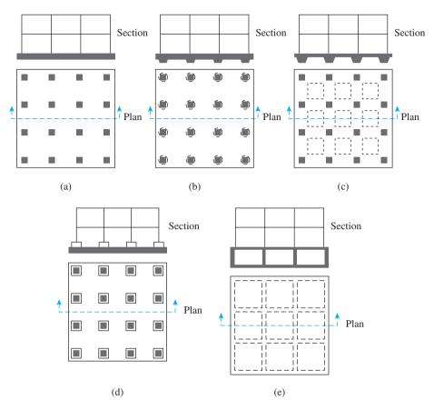
Figure 8.4 Common types of mat foundations
