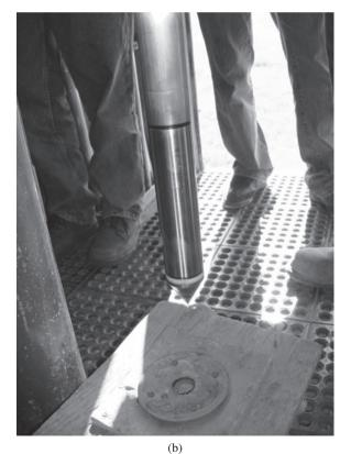
Figure 3.27 Cone penetration test in field: (a) mounted CPT rig; (b) cone penetrometer being set in proper location (Courtesy of Sanjeev Kumar, Southern Illinois University, Carbondale, Illinois)
