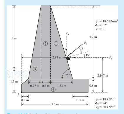
Figure 13.13 Gravity retaining wall (not to scale)
