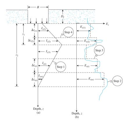
**Figure 7.10** Procedure for calculation of  $S_e$  using the strain influence factor
