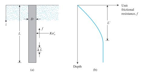
Figure 9.16 Unit frictional resistance for piles in sand
