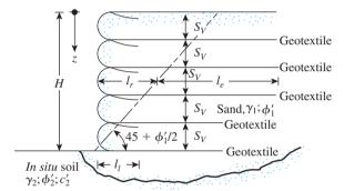
Figure 13.31 Retaining wall with geotextile reinforcement
