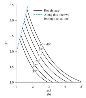
**Figure 5.18** Variation of efficiency ratios with x/B and  $\phi'$
