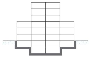
Figure 8.8 Compensated foundation
