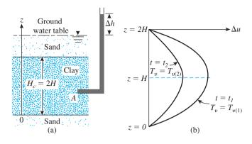
Figure 2.20 (a) Derivation of Eq. (2.72); (b) nature of variation of  $\Delta u$  with time
