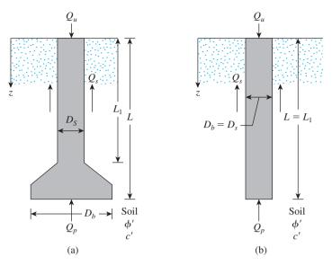
Figure 10.9 Ultimate bearing capacity of drilled shafts: (a) with bell and (b) straight shaft
