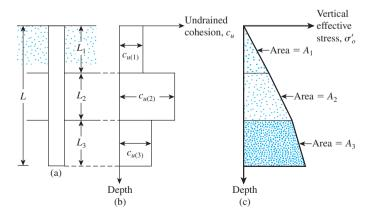
**Figure 9.20** Application of  $\lambda$  method in layered soil
