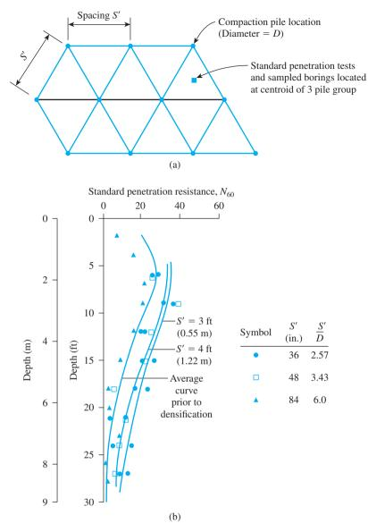
Figure 16.37 Sand compaction pile test of Basore and Boitano (1969): (a) layout of the compaction piles; (b) standard penetration resistance variation with depth and S'
