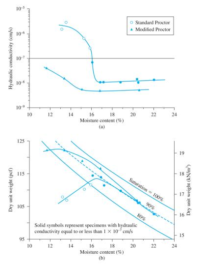
Figure 16.6 Standard and Modified Proctor test results and hydraulic conductivity of Wisconsin A soil (Based on Othman, M. A., and S. M. Luettich, "Compaction Control Criteria for Clay Hydraulic Barriers," Transportation Research Record 1462, Transportation Research Board, National Research Council, Washington, D.C., 1994.)
