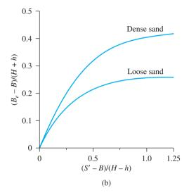
Figure 14.40 (a) Actual case for row of anchors; (b) variation of  $(B_e - B)/(H + h)$ with (S' - B)/(H + h) (Based on Ovesen and Stromann, 1972)
