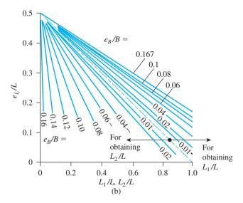
**Figure 4.26** Effective area for the case of  $e_L/L < 0.5$  and  $0 < e_B/B < \frac{1}{6}$  (After Highter and Anders, 1985) (Based on Highter, W. H. and Anders, J. C. (1985). "Dimensioning Footings Subjected to Eccentric Loads," Journal of Geotechnical Engineering, American Society of Civil Engineers, Vol. 111, No. GT5, pp. 659-665.)
