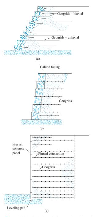
Figure 13.36 Typical schematic diagrams of retaining walls with geogrid reinforcement: (a) geogrid wraparound wall; (b) wall with gabion facing; (c) concrete panel-faced wall (Based on Berg et al., 1986)
