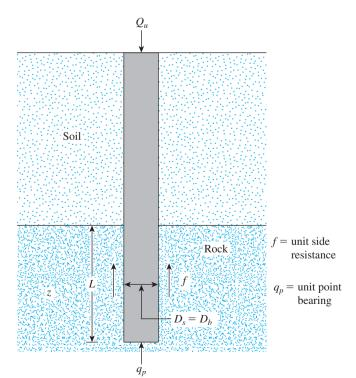
Figure 10.26 Drilled shaft socketed into rock
