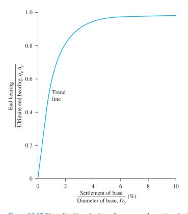
Figure 10.17 Normalized base-load transfer versus settlement in cohesive soil
