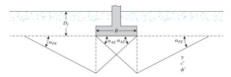
Figure 5.27 Failure surface in soil for seismic bearing-capacity analysis
