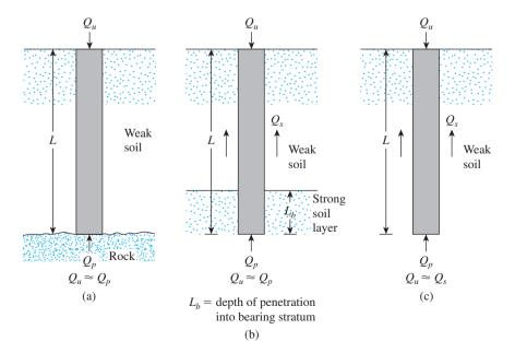
Figure 9.6 (a) and (b) Point bearing piles; (c) friction piles
