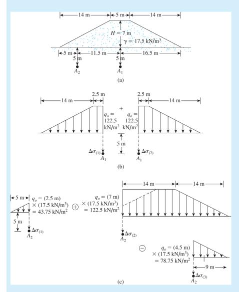
Figure 6.19 Stress increase due to embankment loading
