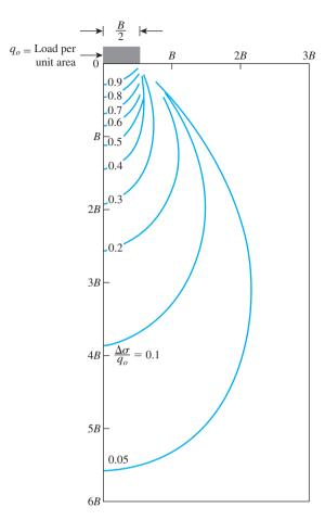
**Figure 6.8** Contours of  $\Delta \sigma/q_o$ below a strip load
