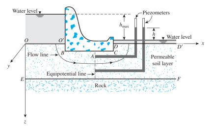
Figure 2.11 Steady-state seepage
