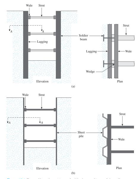
Figure 15.1 Types of braced cut: (a) use of soldier beams; (b) use of sheet piles
