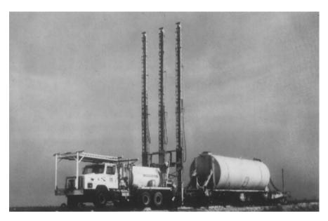
Figure 16.30 Equipment for pressure injection of lime slurry (Courtesy of Hayward Baker Inc., Odenton, Maryland)
