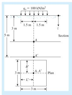
Figure 6.14 Determination of average increase in stress below a rectangular area
