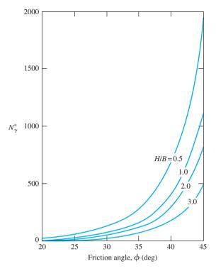
Figure 5.7 Cerato and Lutenegger's test results for  $N_{\gamma}^*$
