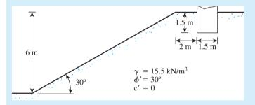
Figure 5.22 Foundation on a granular slope
