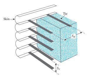
Figure 13.23 Reinforced-earth retaining wall
