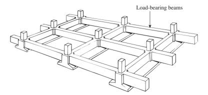
Figure 11.6 Continuous foundation with load-bearing beams (Based on data from Clemence, S. P., and Finbarr, A. O. (1981). "Design Considerations for Collapsible Soils," Journal of the Geotechnical Engineering Division, American Society of Civil Engineers, Vol. 107, GT3 pp. 305–317.)
