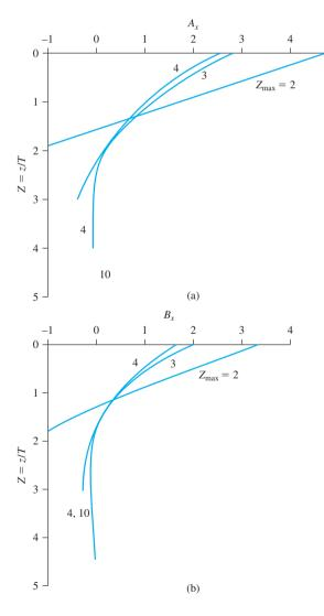
*Figure 9.33* Variation of  $A_x$ ,  $B_x$ ,  $A_m$ , and  $B_m$  with Z (Based on Matlock, H. and Reese, L. C. (1960). "Generalized Solution for Laterally Loaded Piles," *Journal of the Soil Mechanics and Foundations Division*, American Society of Civil Engineers, Vol. 86, No. SM5, Part I, pp. 63–91.)
