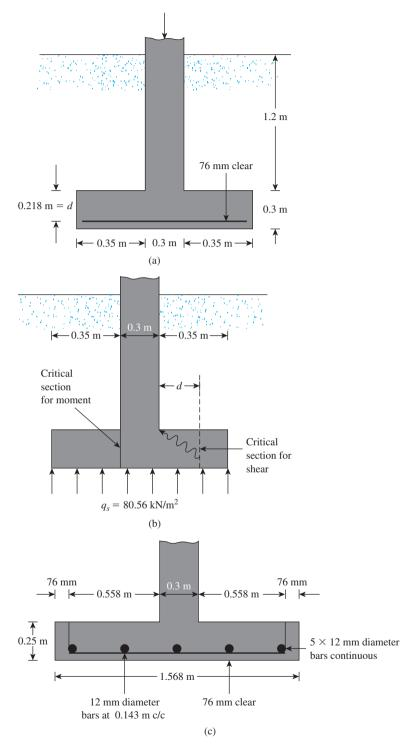
Figure A.2 Continuous wall foundation
