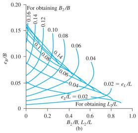
Figure 4.28 Effective area for the case of  $e_L/L < \frac{1}{6}$  and  $e_B/B < \frac{1}{6}$  (Based on Highter, W. H. and Anders, J. C. (1985). "Dimensioning Footings Subjected to Eccentric Loads," Journal of Geotechnical Engineering, American Society of Civil Engineers, Vol. 111, No. GT5, pp. 659–665.)
