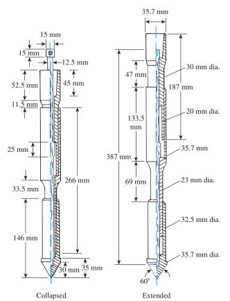
Figure 3.24 Mechanical friction-cone penetrometer (After ASTM, 2001) (Based on Annual Book of ASTM Standards, Vol. 04.08.)
