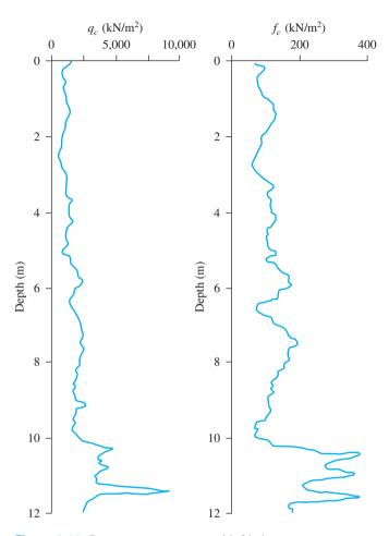
Figure 3.28 Cone penetrometer test with friction measurement
