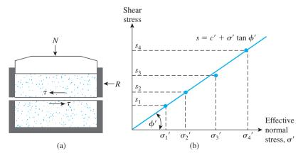
**Figure 2.26** Direct shear test in sand: (a) schematic diagram of test equipment; (b) plot of test results to obtain the friction angle  $\phi'$
