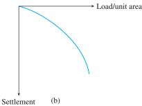
Figure 7.25 Plate load test: (a) test arrangement; (b) nature of load-settlement curve
