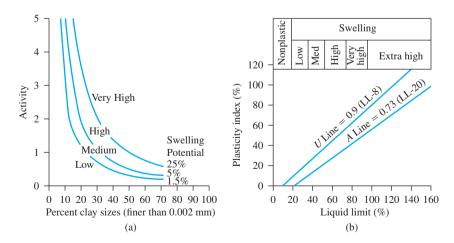
*Figure 11.19* Commonly used criteria for determining swell potential (Based on Abduljauwad, S. N. and Al-Sulaimani, G. J. (1993). "Determination of Swell Potential of Al-Qatif Clay," *Geotechnical testing Journal*, American Society for Testing and Materials, Vol. 16, No. 4, pp. 469–484.)
