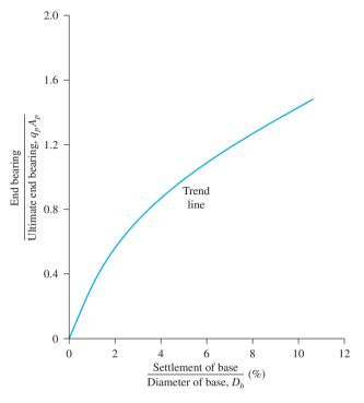
Figure 10.11 Normalized base-load transfer versus settlement in sand
