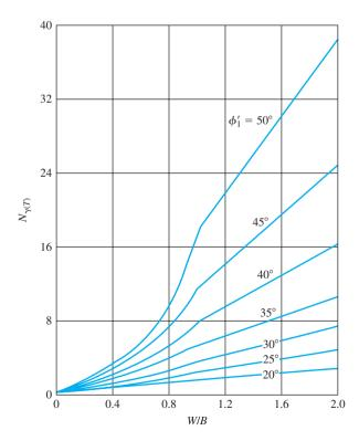
Figure 5.16 Madhav and Vitkar's bearing-capacity factor  $N_{\gamma(T)}$
