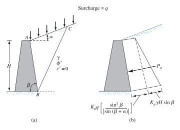
Figure 12.13 Coulomb's active pressure with a surcharge on the backfill
