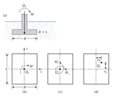
Figure 4.24 Analysis of foundation with two-way eccentricity
