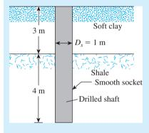
Figure 10.28 Drilled shaft extending into rock
