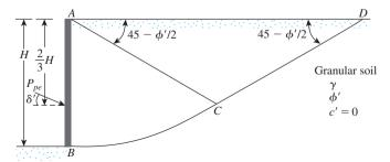
Figure 12.25 Nature of failure surface in soil considered in the analysis to determine  $P_{pe}$
