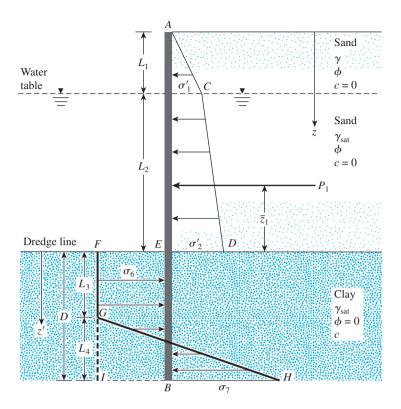
Figure 14.13 Cantilever sheet pile penetrating clay
