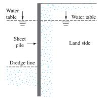
Figure 14.1 Example of waterfront sheet-pile wall
