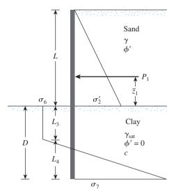
Figure 14.15 Sheet-pile wall penetrating clay
