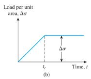
*Figure 2.23* One-dimensional consolidation due to single ramp loading
