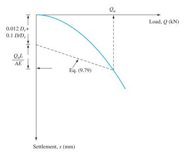
**Figure 9.28** Davisson's method for determination of  $Q_u$
