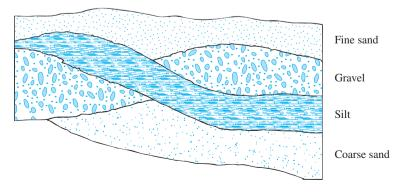
Figure 3.3 Cross section of a braided-stream deposit
