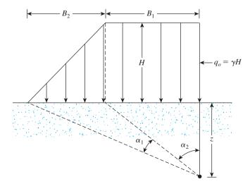
Figure 6.17 Embankment loading
