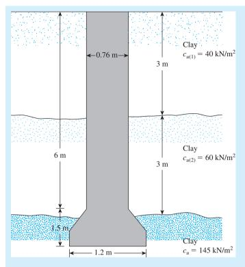
Figure 10.19 A drilled shaft in layered clay
