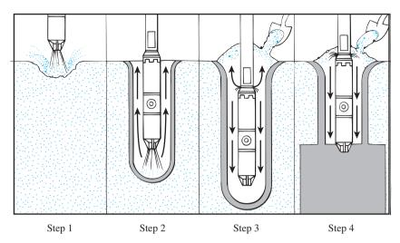
Figure 16.11 Compaction by the vibroflotation process (Based on Brown, 1977.)
