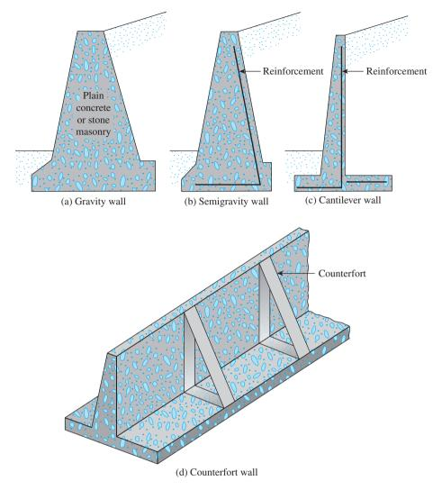
Figure 13.1 Types of retaining wall
