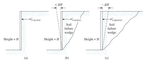
Figure 12.1 Nature of lateral earth pressure on a retaining wall
