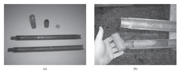
Figure 3.16 (a) Unassembled split-spoon sampler; (b) after sampling (Courtesy of Professional Service Industries, Inc. (PSI), Waukesha, Wisconsin)
