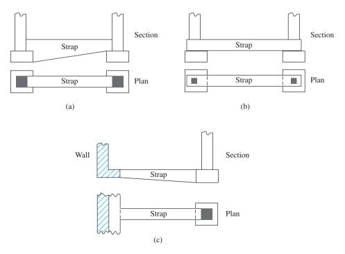
Figure 8.3 Cantilever footing—use of strap beam
