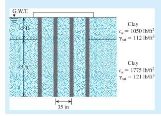
Figure 9.49 Group pile of layered saturated clay
