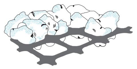
Figure 13.21 Geogrid apertures allowing interlocking with surrounding soil
