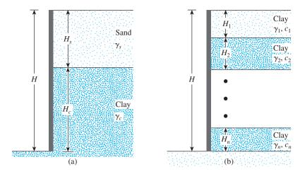
Figure 15.10 Layered soils in braced cuts
