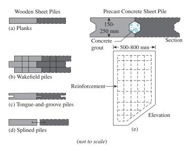
Figure 14.2 Various types of wooden and concrete sheet pile
