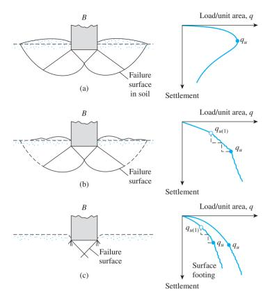
Figure 4.1 Nature of bearing capacity failure in soil: (a) general shear failure: (b) local shear failure; (c) punching shear failure (Redrawn after Vesic, 1973) (Based on Vesic, A. S. (1973). "Analysis of Ultimate Loads of Shallow Foundations," *Journal of Soil Mechanics and Foundations Division*, American Society of Civil Engineers, Vol. 99, No. SM1, pp. 45–73.)
