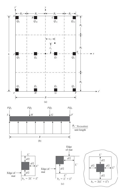
Figure 8.10 Conventional rigid mat foundation design
