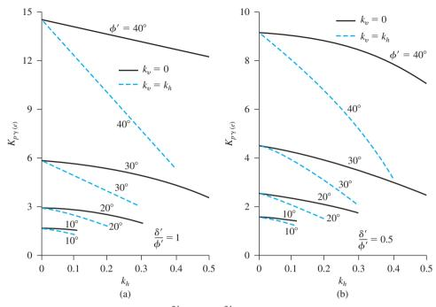
**Figure 12.26** Variation of  $K_{p\gamma(e)}$ : (a)  $\frac{\delta'}{\phi'} = 1$ ; (b)  $\frac{\delta'}{\phi'} = 0.5$
