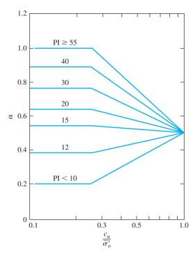
**Figure 9.21** Variation of  $\alpha$  with  $c_u/\overline{\sigma}'_o$ for the NGI-99 method [Eqs. (9.57a) and (9.57b)]
