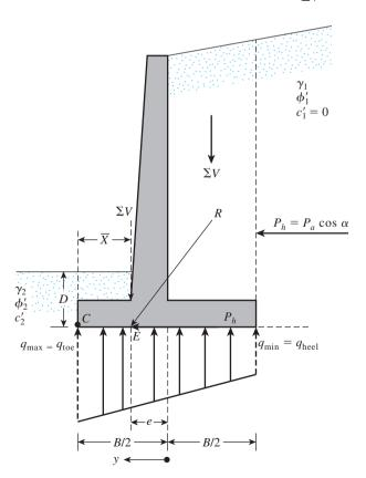
Figure 13.11 Check for bearing capacity failure
