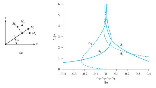
Figure 8.13 Approximate flexible method of mat design
