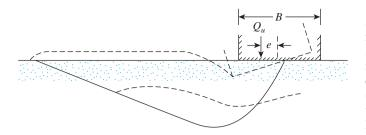
Figure 4.18 Nature of failure surface in soil supporting a strip foundation subjected to eccentric loading (Note:  $D_f = 0$ ;  $Q_u$  is ultimate load per unit length of foundation)
