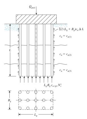
Figure 9.47 Ultimate capacity of group piles in clay
