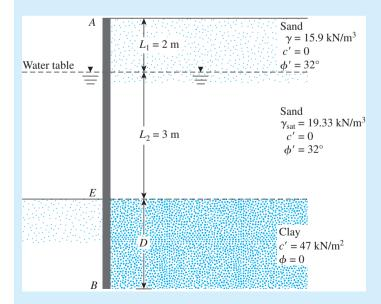
Figure 14.14 Cantilever sheet pile penetrating into saturated clay
