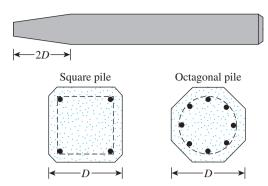
Figure 9.3 Precast piles with ordinary reinforcement
