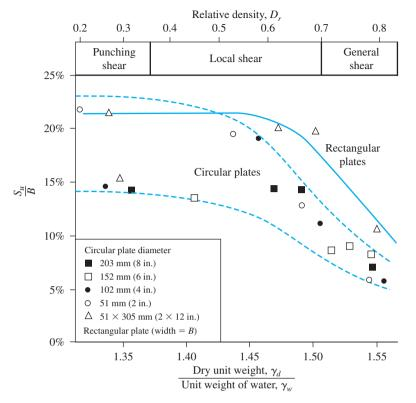
**Figure 4.4** Range of settlement of circular and rectangular plates at ultimate load  $(D_f/B=0)$  in sand (Modified from Vesic, 1963) (Based on Vesic, A. B. Bearing Capacity of Deep Foundations in Sand. In Highway Research Record 39, Highway Research Board, National Research Council, Washington, D.C., 1963, Figure 29, p. 138.)
