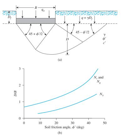
**Figure 5.1** (a) Failure surface under a rough continuous foundation; (b) variation of D/B with soil friction angle  $\phi'$
