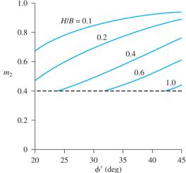
**Figure 5.6** Variation of  $m_1$  and  $m_2$ with H/B and  $\phi'$
