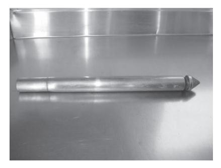
Figure 3.26 Photograph of an electric friction-cone penetrometer (Courtesy of Sanjeev Kumar, Southern Illinois University, Carbondale, Illinois)
