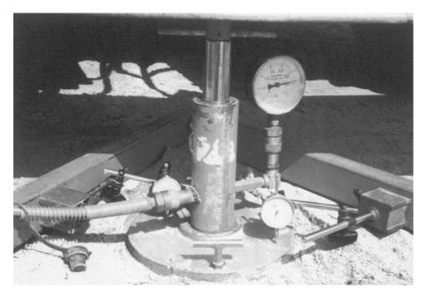
Figure 7.26 Plate load test in the field (Courtesy of Braja M. Das, Henderson, Nevada)
