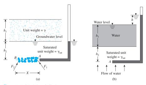
Figure 2.13 Calculation of effective stress
