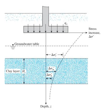
Figure 7.20 Consolidation settlement calculation
