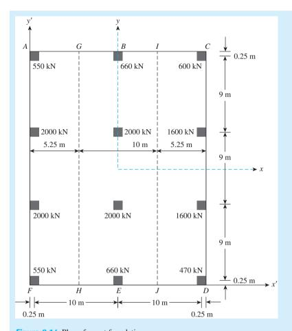
Figure 8.14 Plan of a mat foundation
