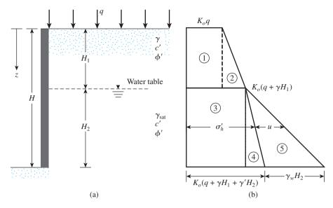
**Figure 12.4** At-rest earth pressure with water table located at a depth z < H
