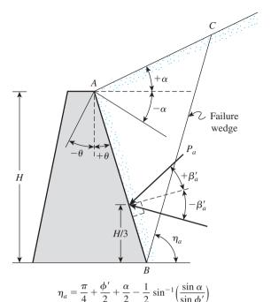
Figure 12.9 Location and direction of Rankine active force
