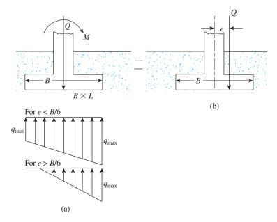
Figure 4.17 Eccentrically loaded foundations
