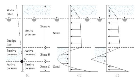
Figure 14.8 Cantilever sheet pile penetrating sand
