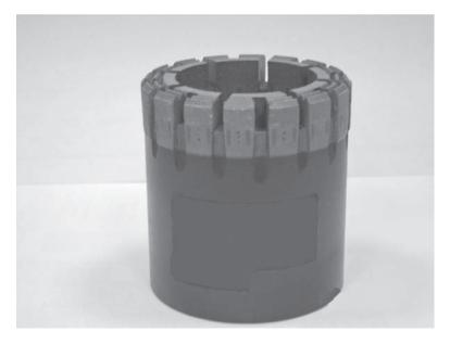
Figure 3.42 Diamond coring bit (Courtesy of Braja M. Das, Henderson, Nevada)
