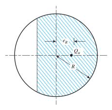
Figure 4.29 Effective area for circular foundation
