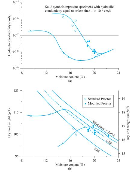
Figure 16.7 Standard and Modified Proctor test results and hydraulic conductivity of Wisconsin B soil (Based on Othman, M. A., and S. M. Luettich, "Compaction Control Criteria for Clay Hydraulic Barriers," Transportation Research Record 1462, Transportation Research Board, National Research Council. Washington, D.C., 1994.)
