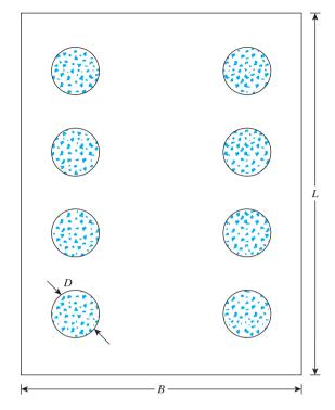
Figure 16.35 Shallow foundation over a group of stone columns
