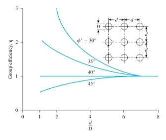
**Figure 9.46** Variation of efficiency of pile groups in sand (Based on Kishida and Meyerhof, 1965)
