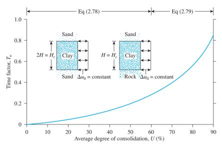
**Figure 2.22** Plot of time factor against average degree of consolidation ( $\Delta u_0 = \text{constant}$ )
