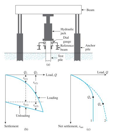
Figure 9.27 (a) Schematic diagram of pile load test arrangement; (b) plot of load against total settlement; (c) plot of load against net settlement
