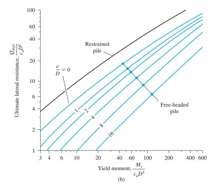
Figure 9.36 Broms's solution for ultimate lateral resistance of long piles (a) in sand (b) in clay
