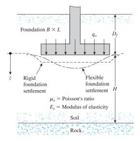
Figure 7.3 Elastic settlement of flexible and rigid foundations
