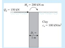
Figure 10.25 Free-headed drilled shaft
