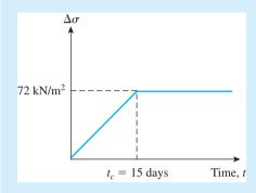
Time, t Figure 2.25 Ramp loading
