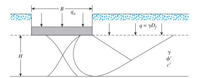
*Figure 5.2* Failure surface under a rough, continuous foundation with a rigid, rough base located at a shallow depth
