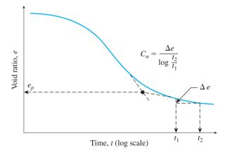
**Figure 7.24** Variation of *e* with log t under a given load increment, and definition of secondary compression index
