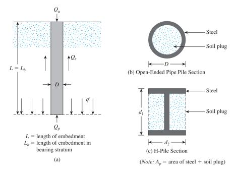
Figure 9.11 Ultimate load-carrying capacity of pile
