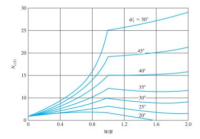
**Figure 5.14** Madhav and Vitkar's bearing-capacity factor  $N_{c(T)}$
