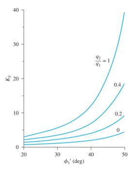
Figure 5.10 Meyerhof and Hanna's punching shear coefficient  $K_s$
