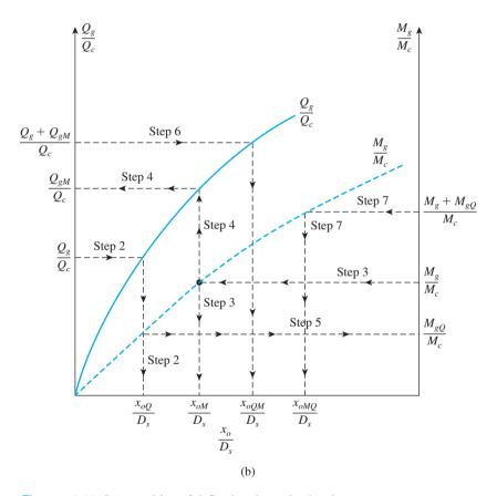
Figure 10.22 Superposition of deflection due to load and moment
