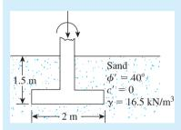
Figure 4.23 A continuous foundation with load eccentricity
