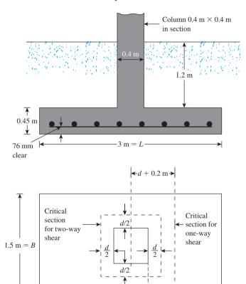
Figure A.4 Rectangular foundation for a column
