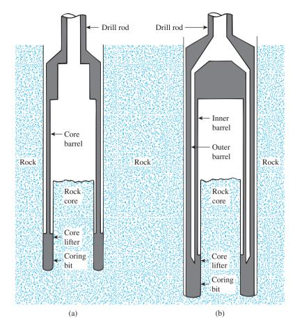
Figure 3.41 Rock coring: (a) single-tube core barrel; (b) double-tube core barrel
