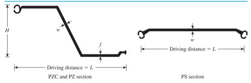
the steel sheet-pile sections produced by Hammer & Steel, Inc. of Hazelwood, Missouri. The allowable design flexural stress for the steel sheet piles is as follows:
