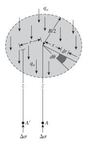
Figure 6.2 Increase in pressure under a uniformly loaded flexible circular area
