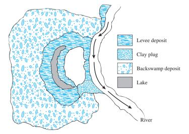
Figure 3.5 Levee and backswamp deposit
