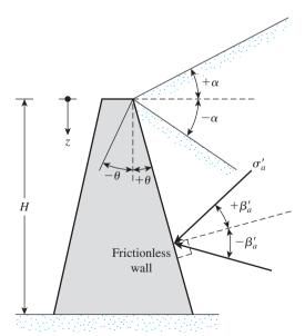
Figure 12.8 General case for a retaining wall with granular backfill
