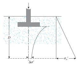
Figure 3.9 Determination of the minimum depth of boring
