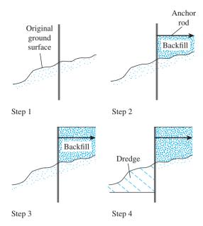
Figure 14.7 Sequence of construction for a dredged structure
