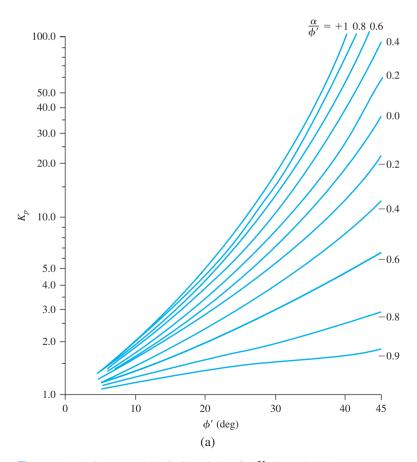
**Figure 12.24** Caquot and Kerisel's solution for  $K_p$  [Eq.(12.70)]
