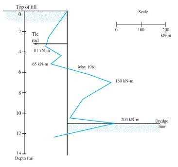
Figure 14.31 Bending moment from straingage measurements at test location 3, Toledo bulkhead (Based on Casagrande, 1973)
