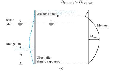
Figure 14.17 Nature of variation of deflection and moment for anchored sheet piles: (a) free earth support method
