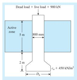
Figure 11.27 Drilled shaft in a swelling clay
