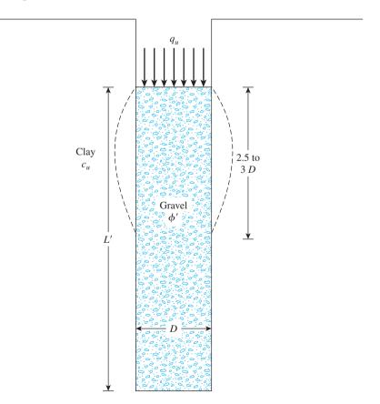
Figure 16.34 Bearing capacity of stone column
