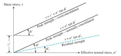
Figure 2.33 Peak- and residual-strength envelopes for clay
