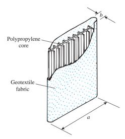
Figure 16.25 Prefabricated vertical drain (PVD)
