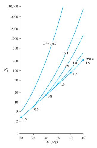
Figure 5.5 Mandel and Salencon's bearing capacity factor  $N_{\gamma}^*$  [Eq. (5.2)]
