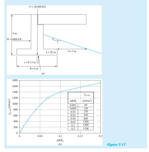
acts on the foundation. The active pressure on the abutment wall develops a 1,600 kN horizontal load. The resultant reaction force due to the vertical and horizontal load is applied at an eccentricity of 0.13 m. PMT testing at the site produced a mean Pressuremeter curve characterizing the soil and is shown in Figure 7.17b. What is the settlement at the current loading?
