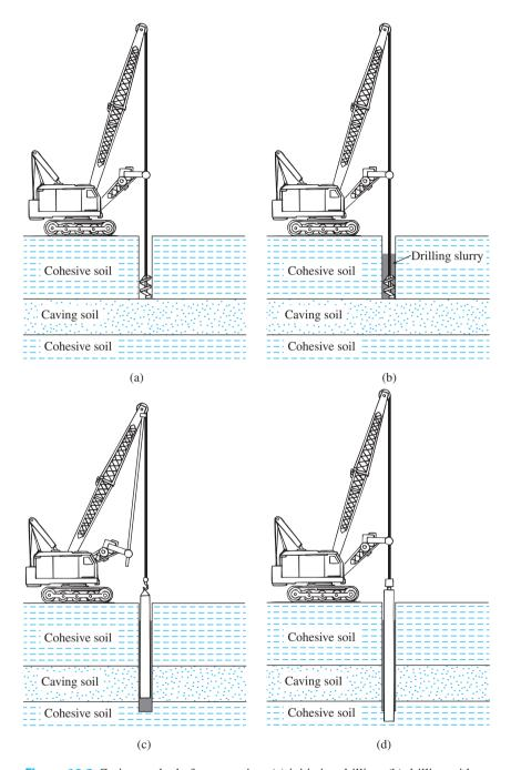
Figure 10.3 Casing method of construction: (a) initiating drilling; (b) drilling with slurry; (c) introducing casing; (d) casing is sealed and slurry is being removed from interior of casing; (e) drilling below casing; (f) underreaming; (g) removing casing; (h) completed shaft (Based on O'Neill and Reese, 1999)
