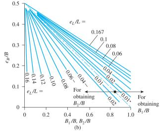
**Figure 4.27** Effective area for the case of  $e_L/L < \frac{1}{6}$  and  $0 < e_B/B < 0.5$  (Based on Highter, W. H. and Anders, J. C. (1985). "Dimensioning Footings Subjected to Eccentric Loads," Journal of Geotechnical Engineering, American Society of Civil Engineers, Vol. 111, No. GT5, pp. 659–665.)
