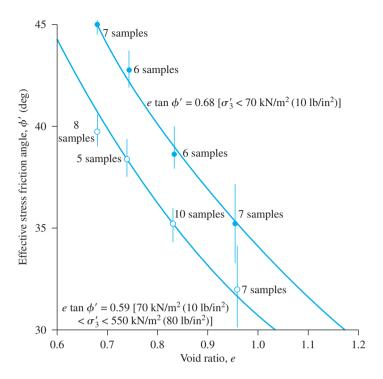
**Figure 2.30** Variation of friction angle  $\phi'$  with void ratio for Chattachoochee River sand (After Vesic, 1963) (Based on Vesic, A.B. Bearing Capacity of Deep Foundations in Sand. In *Highway Research Record 39*, Highway Research Board. National Research Council, Washington, D.C., 1963, Figure 11, p. 123.)
