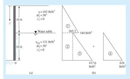
Figure 12.7 Rankine active force behind a retaining wall
