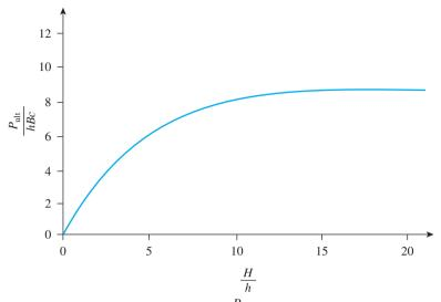
**Figure 14.44** Experimental variation of  $\frac{P_{\text{ult}}}{hBc}$  with H/h for plate anchors in clay (Based on Mackenzie (1955) and Tschebotarioff (1973))
