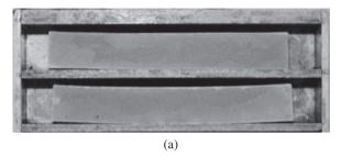
Figure 11.21 Shrinkage of expansive clay (Eagle Ford soil) mixed with water to about its liquid limit in molds of 152 mm × 12.7 mm × 12.7 mm (6 in. × ½ in. × ½ in.): (a) without addition of lime; (b) with addition of 6% lime by weight (Courtesy of Thomas M. Petry, Missouri University of Science and Technology, Rolla, Missouri)
