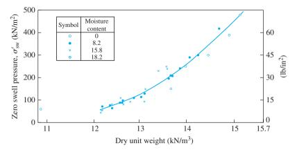
*Figure 11.16* Plot of zero swell pressure with the dry unit weight of soil (Based on Sridharan et al., 1986.)
