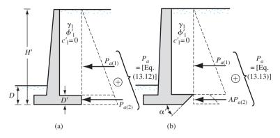
Figure 13.10 Retaining wall with sloped heel
