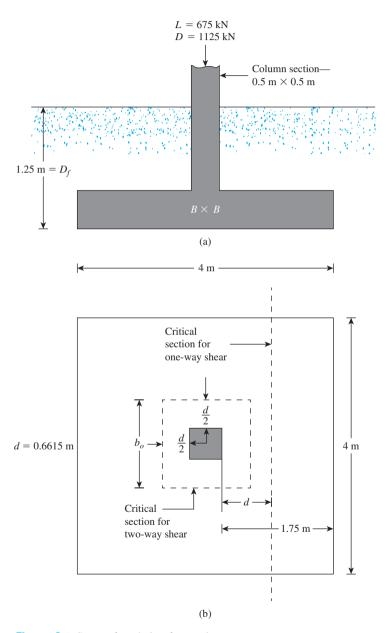
Figure A.3 Square foundation for a column
