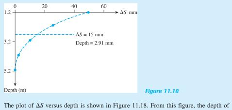
undercut is 2.91 - 1.2 = 1.71 m below the bottom of the foundation.
