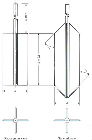
Figure 3.23 Geometry of field vane (After ASTM, 2014) (Based on Annual Book of ASTM Standards, Vol. 04.08.)
