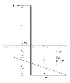
Figure 14.16 Free cantilever sheet piling penetrating clay
