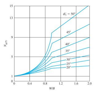
Figure 5.15 Madhav and Vitkar's bearing-capacity factor  $N_{q(T)}$
