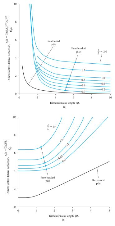
Figure 9.37 Broms's solution for estimating deflection of pile head (a) in sand and (b) in clay
