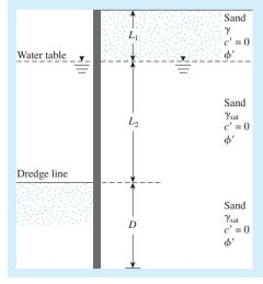
Figure 14.10 Cantilever sheet-pile wall
