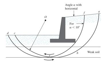
*Figure 13.6* Deep-seated shear failure
