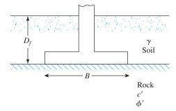
Figure 5.32 Foundation on rock
