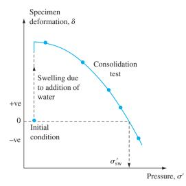
**Figure 11.14** Zero swell pressure from conventional consolidation test
