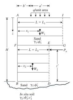
Figure 13.29 Stability check for the retaining wall
