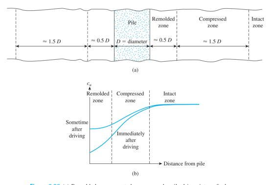
Figure 9.29 (a) Remolded or compacted zone around a pile driven into soft clay; (b) Nature of variation of undrained shear strength  $(c_u)$  with time around a pile driven into soft clay
