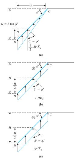
**Figure 4.8** Passive force distribution on the wedge face *CD* shown in Figure 4.7:
