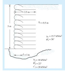
Figure 13.34 Geotextile-reinforced retaining wall
