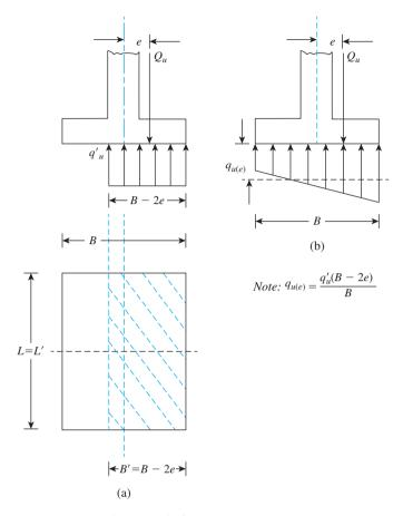
**Figure 4.19** Definition of  $q'_u$  and  $q_{u(e)}$
