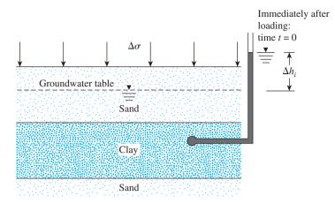
Figure 2.15 Principles of consolidation
