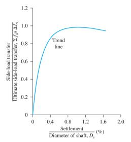
Figure 10.12 Normalized side-load transfer versus settlement in sand
