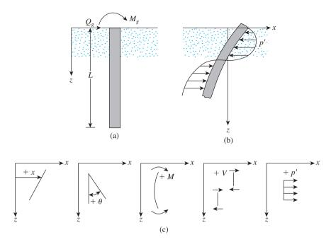
Figure 9.32 (a) Laterally loaded pile; (b) soil resistance on pile caused by lateral load; (c) sign conventions for displacement, slope, moment, shear, and soil reaction
