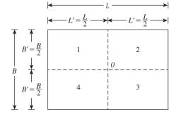
Figure 6.13 Average stress increase calculation below a flexible loaded rectangular area
