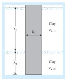
Figure 10.18 A drill shaft without a bell
