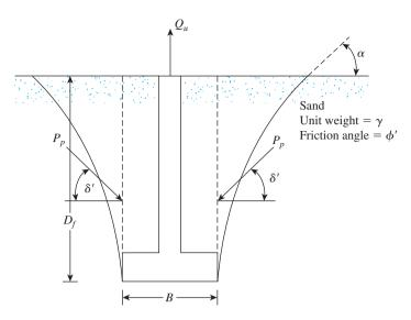
Figure 5.33 Shallow continuous foundation subjected to uplift
