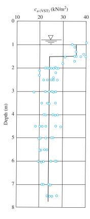
**Figure 4.14** Variation of  $c_{u(VST)}$  with depth for soft Bangkok clay
