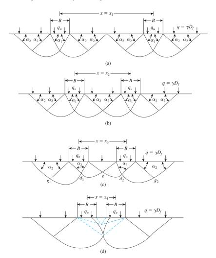
Figure 5.17 Assumptions for the failure surface in granular soil under two closely spaced rough continuous foundations
