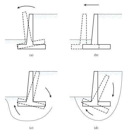
Figure 13.5 Failure of retaining wall:
