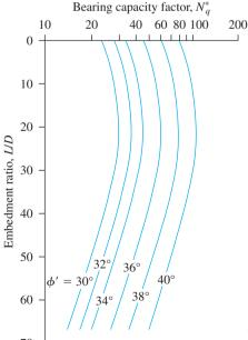
**Figure 9.15** Variation of  $N_q^*$  with L/D(Based on Coyle and Costello, 1981)
