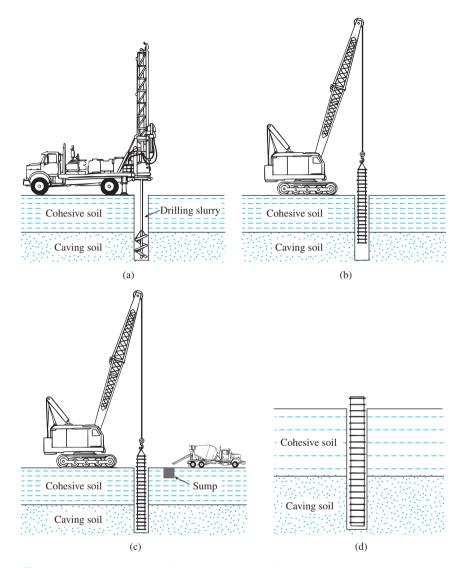
Figure 10.4 Slurry method of construction: (a) drilling to full depth with slurry; (b) placing rebar cage; (c) placing concrete; (d) completed shaft (After O'Neill and Reese, 1999)
