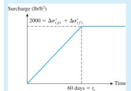
Figure 16.24 Ramp load for a sand drain project
