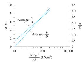
**Figure 16.39** Plot of a/D and b/Dversus  $NW_H h/Ab$  (Based on Poran and Rodriguez, 1992) (Poran, C. J. and Rodriguez, J. A. (1992). "Design of Dynamic Compaction," Canadian Geotechnical Journal, Vol. 29, No. 5, pp. 796-802.)
