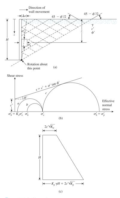
Figure 12.19 Rankine passive pressure
