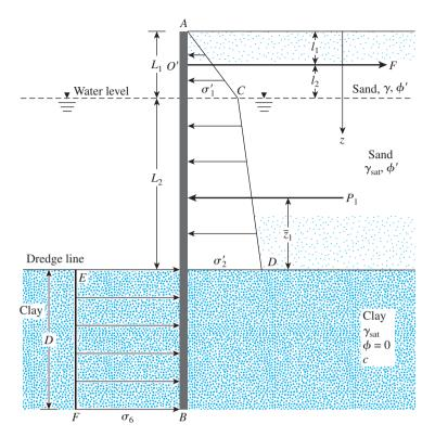
Figure 14.32 Anchored sheet-pile wall penetrating clay
