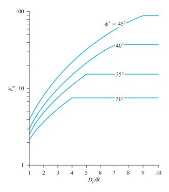
*Figure 5.34* Variation of  $F_a$ with  $D_f/B$  and  $\phi'$
