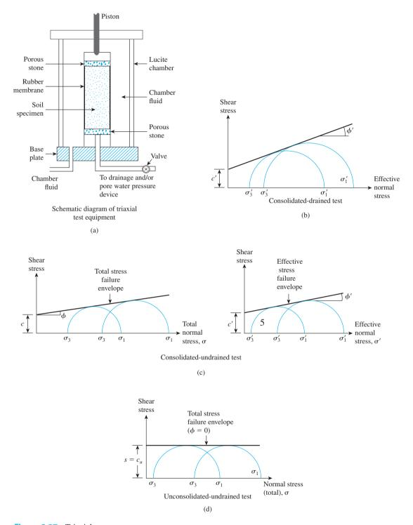
Figure 2.27 Triaxial test
