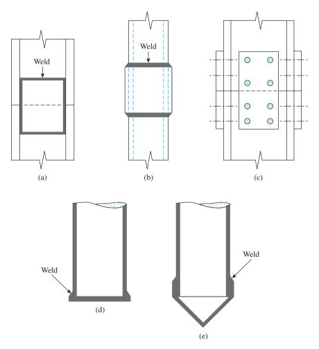
**Figure 9.2** Steel piles: (a) splicing of H-pile by welding; (b) splicing of pipe pile by welding; (c) splicing of H-pile by rivets and bolts; (d) flat driving point of pipe pile; (e) conical driving point of pipe pile
