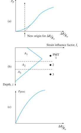
**Figure 7.14** (a) Plot of  $p_p$  versus  $\Delta R/R_o$ ; (b) averaging the pressuremeter curves within the foundation zone of influence; (c) plot of  $p_{p(m)}$  versus  $\Delta R/R_o$
