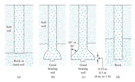
Figure 10.1 Types of drilled shaft: (a) straight shaft; (b) and (c) belled shaft; (d) straight shaft socketed into rock
