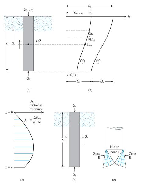
Figure 9.9 Load transfer mechanism for piles
