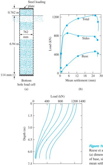
Figure 10.8 Load test results of Reese et al. (1976) on a drilled shaft: (a) dimensions of the shaft; (b) plot of base, sides, and total load with mean settlement; (c) plot of load-distribution curve with depth
