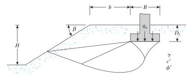
Figure 5.19 Shallow foundation on top of a slope
