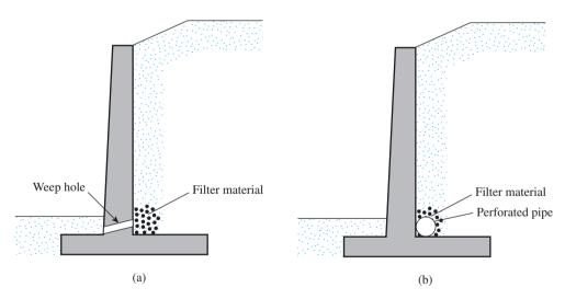
Figure 13.15 Drainage provisions for the backfill of a retaining wall: (a) by weep holes; (b) by a perforated drainage pipe
