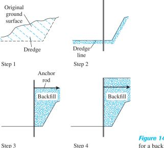
Figure 14.6 Sequence of construction for a backfilled structure
