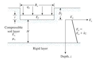
Figure 7.5 Improved equation for calculating elastic settlement: general parameters
