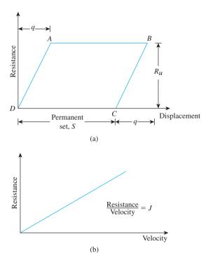
**Figure 9.40** Model for soil–pile interface at pile point: (a) bilinear spring; (b) dashpot
