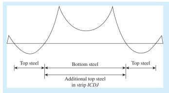
Figure 8.20 General arrangement of reinforcement
