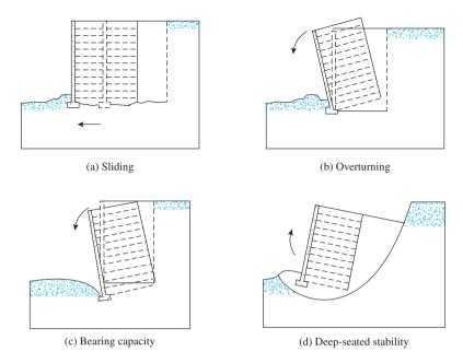
Figure 13.22 External stability checks (After Transportation Research Board, 1995) (Based on Transportation Research Circular 444: Mechanically Stabilized Earth Walls. Transportation Research Board, National Research Council, Washington, D.C., 1995.)
