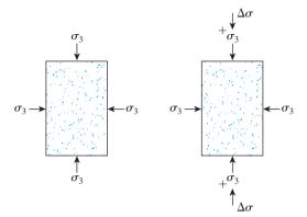
Figure 2.28 Sequence of stress application in triaxial test
