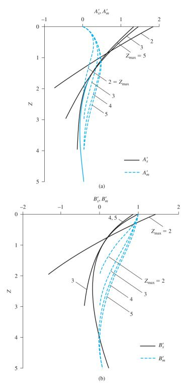
**Figure 9.34** Variation of  $A_x$ ,  $B'_x$ ,  $A'_m$ , and  $B'_m$  with Z (Based on Davisson, M. T. and Gill, H. L. (1963). "Laterally Loaded Piles in a Layered Soil Systems," Journal of the Soil Mechanics and Foundations Division, American Society of Civil Engineers, Vol. 89, No. SM3, pp. 63-94.)
