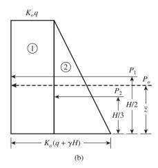
Figure 12.3 At-rest earth pressure
