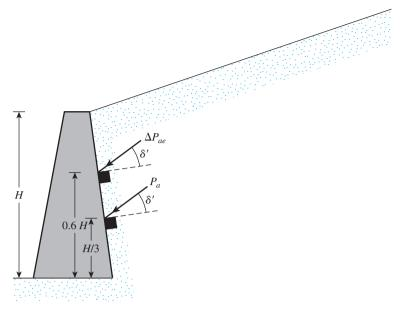
**Figure 12.16** Determining the line of action of  $P_{ae}$
