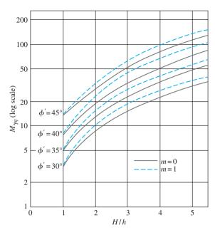
**Figure 14.42** Variation of  $M_{\gamma a}$ with H/h and  $\phi'$  (Based on Neeley et al., 1973.)
