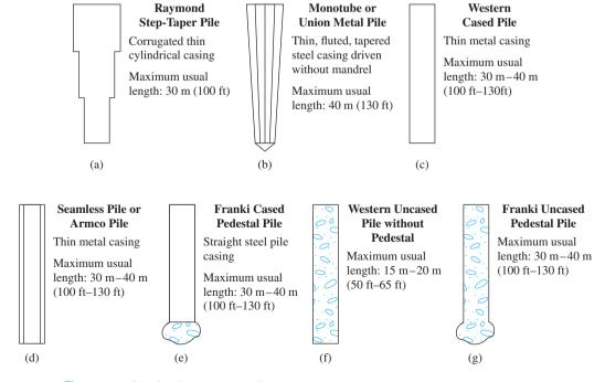
Figure 9.4 Cast-in-place concrete piles
