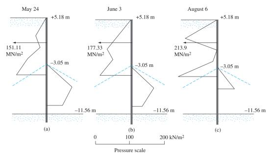
Figure 14.30 Measured stresses at Station 27 + 30—Pier C bulkhead, Long Beach (Based on Casagrande, 1973)
