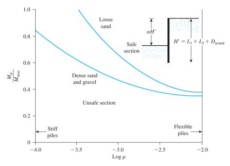
*Figure 14.25* Plot of log  $\rho$  against  $M_d/M_{\rm max}$  for sheet-pile walls penetrating sand (Based on Rowe, P. W. (1952). "Anchored Sheet-Pile Walls," *Proceedings, Institute of Civil Engineers*, Vol. 1, Part 1, pp. 27–70.)
