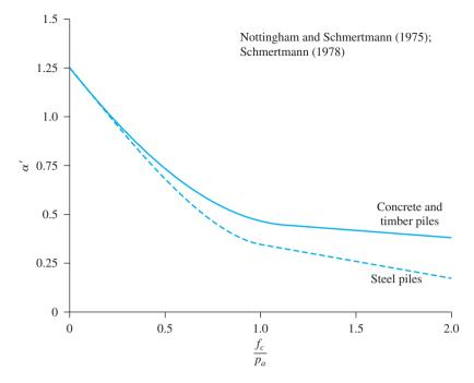
**Figure 9.22** Variation of  $\alpha'$  with  $f_c/p_a$  for piles in clay ( $p_a$  = atmospheric pressure  $\approx 100 \text{ kN/m}^2 \text{ or } 2000 \text{ lb/ft}^2$ )
