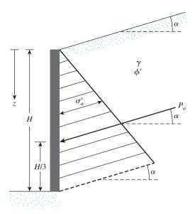
Figure 12.10 Notations for active pressure—Eqs. (12.19), (12.20), (12.21)
