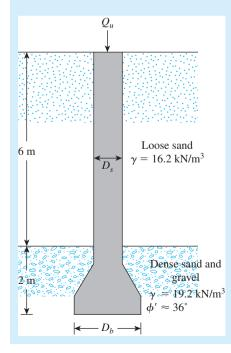
Figure 10.14 Allowable load of drilled shaft
