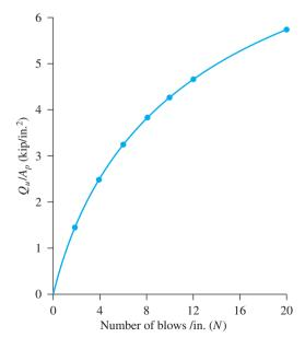
Figure 9.38 Plot of stress versus blows/in.
