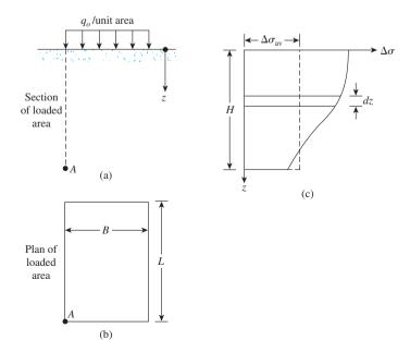
Figure 6.10 Average vertical stress increase due to a rectangularly loaded flexible area
