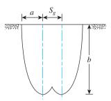
Figure 16.40 Approximate grid spacing for dynamic compaction
