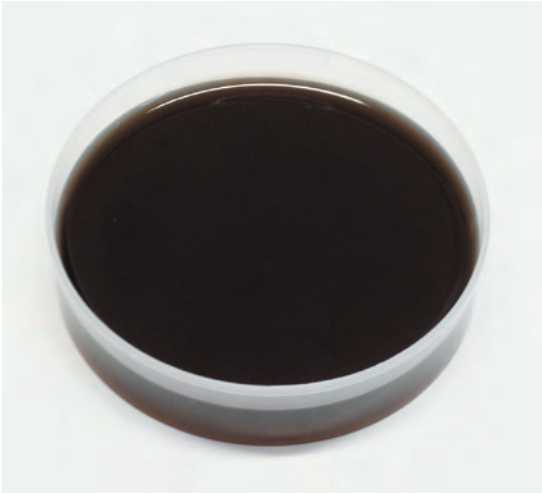
Figure 4.55 Damaged propylene glycol
