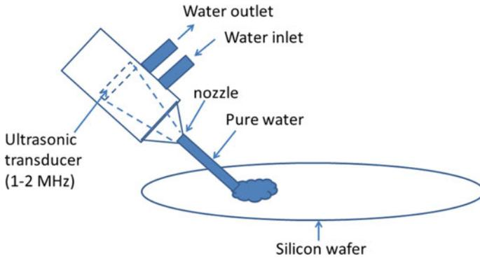
**Fig. 1.25** Ultrasonic spray cleaning
