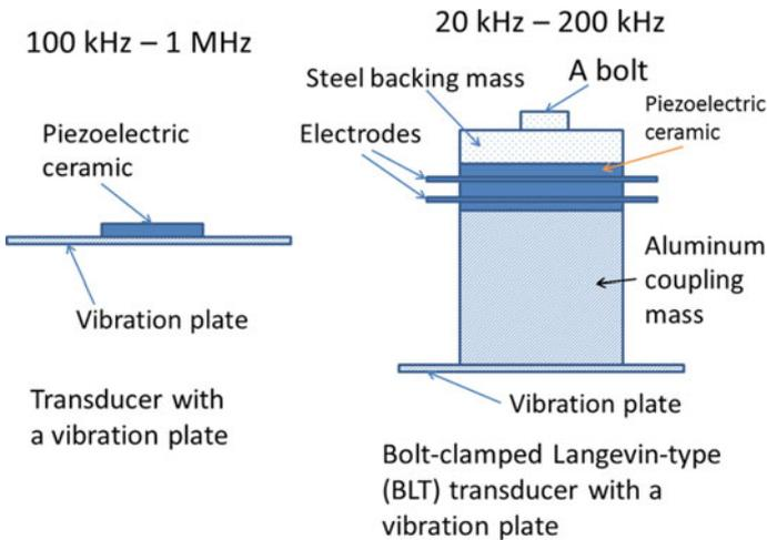
**Fig. 1.4** Typical ultrasonic transducers with a vibration plate
