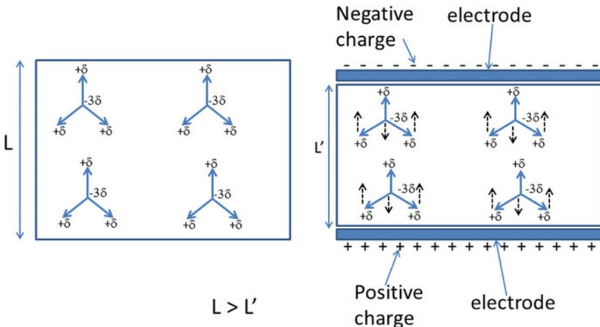
Fig. 1.3 Mechanism of inverse piezoelectric effect
