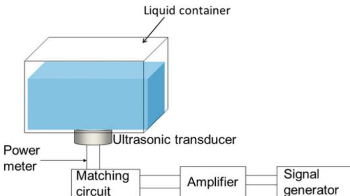
**Fig. 1.7** An electrical drive system for an ultrasonic transducer. Reprinted with permission from Yasui [19]. Copyright (2011), Springer
