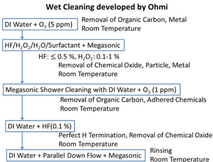
**Fig. 1.26** Wet cleaning developed by Ohmi in 1996 [74]
