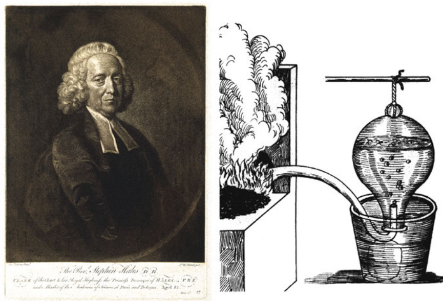
Fig. 1.2 Stephen Hales (1677–1761) at age 82 (Mezzotint by J. McArdeall after T. Hudson, Courtesy of Wellcome Library, London, under Creative Commons Attribution only licence CC BY 4.0) and his pneumatic trough
