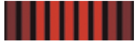
Interference fringes in an optical double-slit interference experiment.
