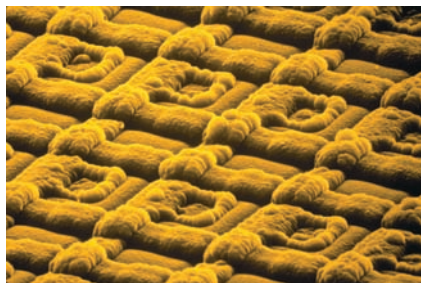
The size of the features in an integrated circuit is limited by the diffraction of light.
