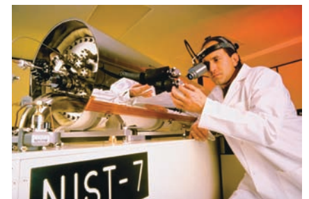
An atomic clock at the National Institute of Standards and Technology is the primary standard of time.
