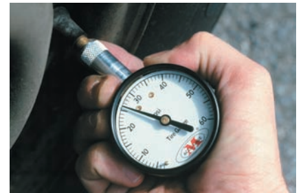
A tire-pressure gauge reads the gauge pressure p_g , not the absolute pressure p .
