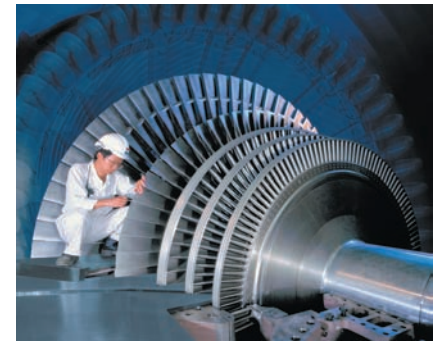
The steam turbine in a modern power plant is an enormous device. Expanding steam does work by spinning the turbine.
