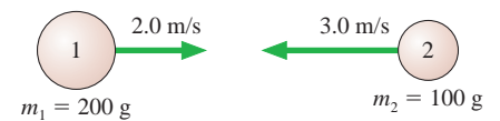
FIGURE 10.34 A perfectly elastic collision in which both balls have an initial velocity.
