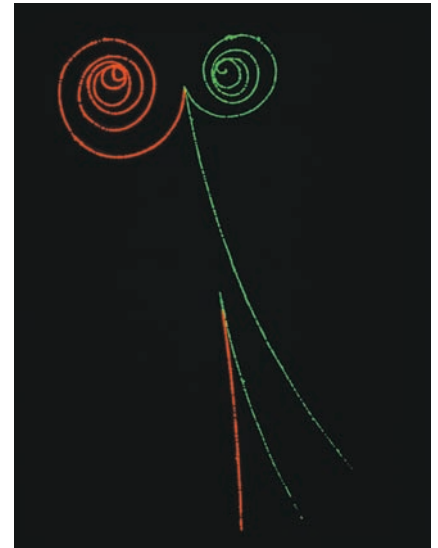
The tracks of elementary particles in a bubble chamber show the creation of an electron-positron pair. The negative electron and positive positron spiral in opposite directions in the magnetic field.
