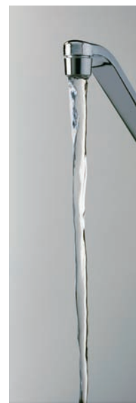
FIGURE 15.29 The flow tube diameter changes as the speed increases. This is a consequence of the equation of continuity.
