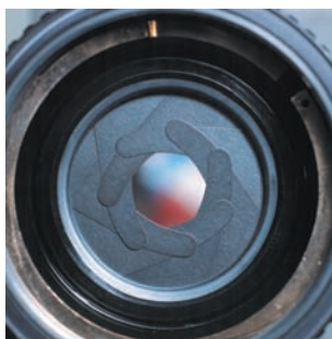
An iris can change the effective diameter of a lens and thus the amount of light reaching the detector.
