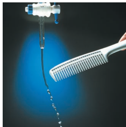
A plastic comb that has been charged by running it through your hair attracts neutral objects—here drops of water.
