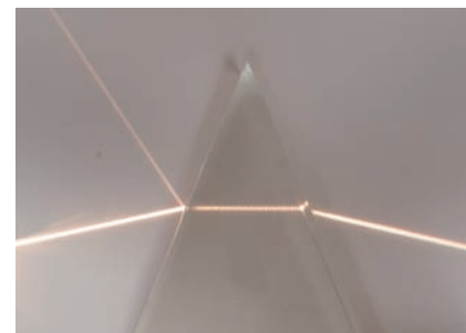
FIGURE 23.13 A light beam refracts twice in passing through a glass prism. You can see a weak reflection from the left surface of the prism.
