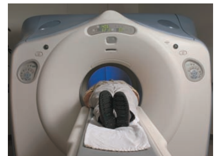
This patient is undergoing magnetic resonance imaging (MRI). The large cylinder surrounding the patient contains a solenoid that is wound with superconducting wire to generate a strong uniform magnetic field.
