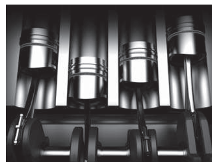
The pistons in a car engine do work on the air-fuel mixture by compressing it.
