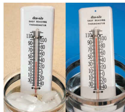
Thermal expansion of the liquid in the thermometer tube pushes it higher in the hot water than in the ice water.
