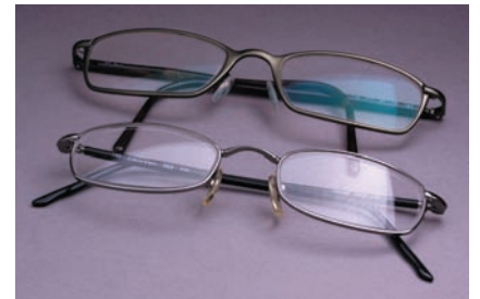
Antireflection coatings use the interference of light waves to nearly eliminate reflections from glass surfaces.
