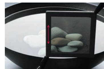
The vertical polarizer blocks the horizontally polarized glare from the surface of the water.
