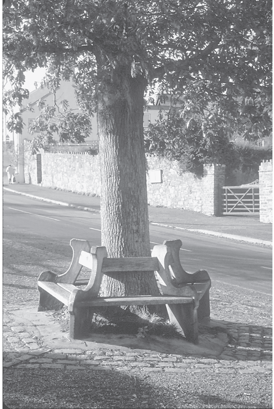
Figure I.15 Sitting under trees seems to be an innate human desire. Furniture or construction under trees must use minimal foundations (if any); erosion from constant use is a concern, but paving is risky unless very porous. (Photo: Kim Sorvig.)
