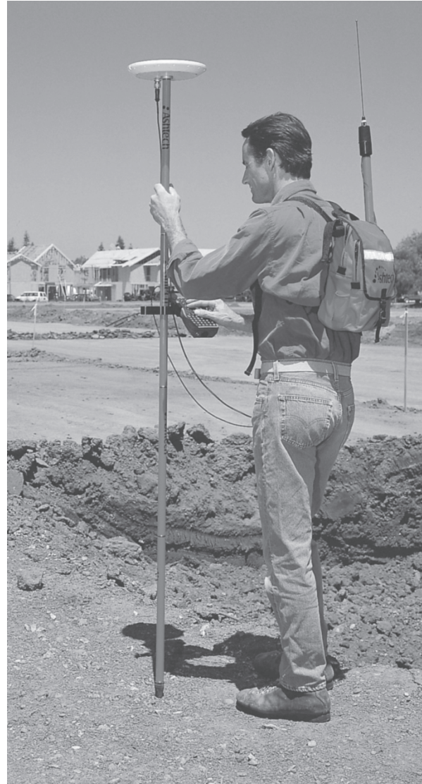
Figure I.4 GPS units, often backpack sized, make surveying quicker, easier, and potentially less destructive to site vegetation, and are an essential part of UAS surveying, below. (Photo: Magellan Corp.)
