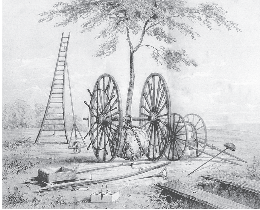
Figure I.18 Col. Greenwood's Treelifter (1844) allowed one worker to transplant a thirty-foot-tall tree. The "ship's wheel" cranked the axle, pulling up the lifting chains. In transit, the axle rotated independently of the chains. ( Illustr. : From "The Tree-Lifter," London, 1844; thanks to Tim Brotzman, Brotzman's Nursery, Madison OH.)
