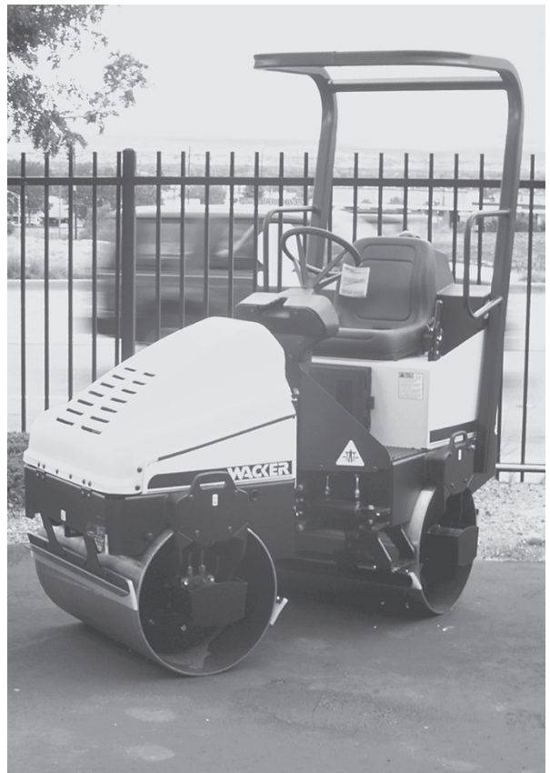
Figure 7.14 Articulated steering, as well as small size, means this roller can work around existing site features instead of obliterating them. (Photo: Kim Sorvig.)
