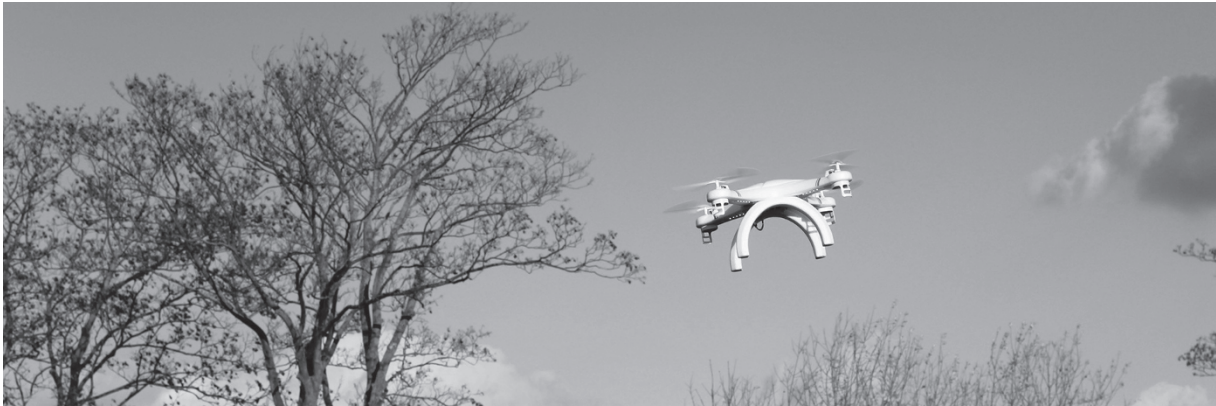
Figure 1.5a, b Unmanned aircraft systems (UAS, or drones) are removing the last excuse for inadequate site data. Fixed-wing ( right ) and rotor types ( below ) make surveying fast and cheap enough for ongoing performance monitoring, and produce 3D models of whole landscapes or specific features. (Photos: Lumpi, Pixabay.)
