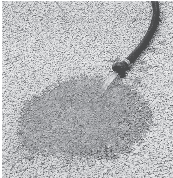
Figure 5.11 Porous concrete, shown here, and porous asphalt support vehicles but permit water to infiltrate rapidly. (Photo: Florida Concrete and Products Association/Dennis Graeber.)
