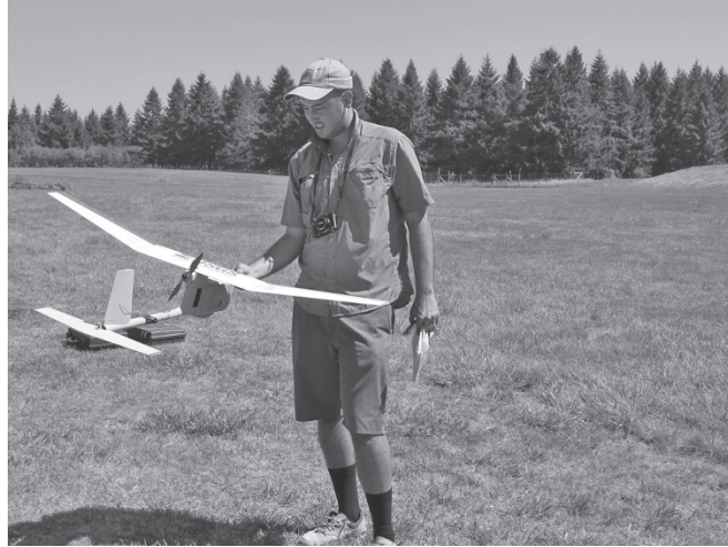
Figure 1.5a, b Unmanned aircraft systems (UAS, or drones) are removing the last excuse for inadequate site data. Fixed-wing ( right ) and rotor types ( below ) make surveying fast and cheap enough for ongoing performance monitoring, and produce 3D models of whole landscapes or specific features. (Photos: Lumpi, Pixabay.)
