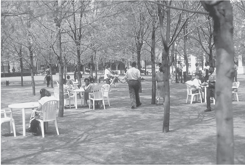
Figure 5.7 Stone screenings over air-entrained soil at MetroTech in Brooklyn create a permeable surface with the feel of traditional French public spaces. (Project and Photo: Henry Arnold.)
