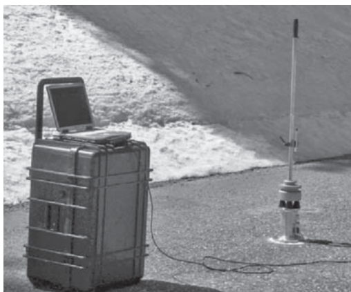
FIGURE 20.3 Portable falling weight deflectometer. (Courtesy of Maureen Kestler/Michael Santi.)
