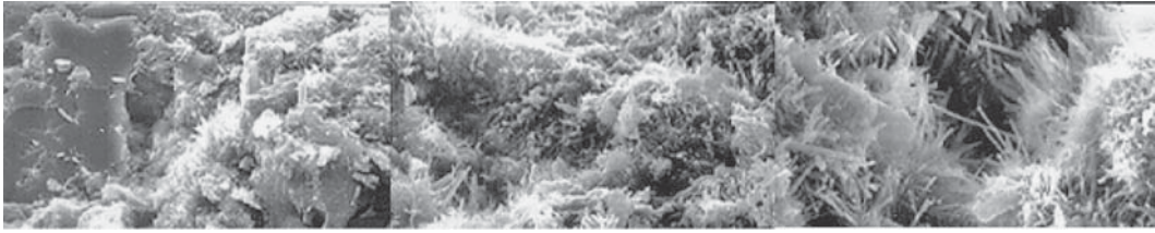
FIGURE 10.3 Scanning electron micrograph showing cement hydration products at various ages; phases include CSH, \text{Ca}(\text{OH})_2 , and Ettringite.
