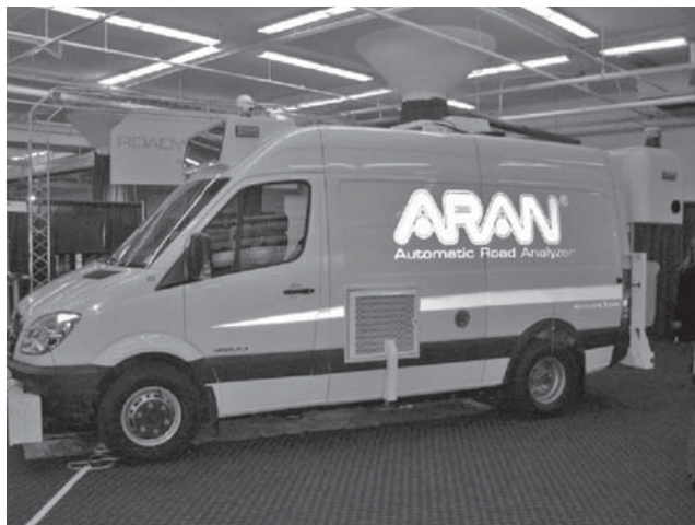
FIGURE 18.3 Automatic road analyzer.
