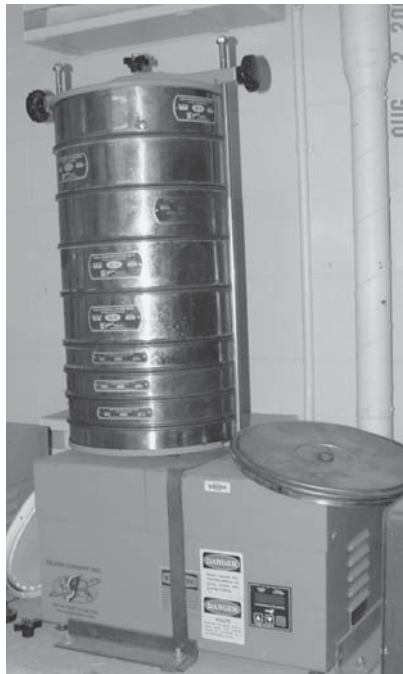
FIGURE 8.4 Stack of sieves in sieve shaker.
