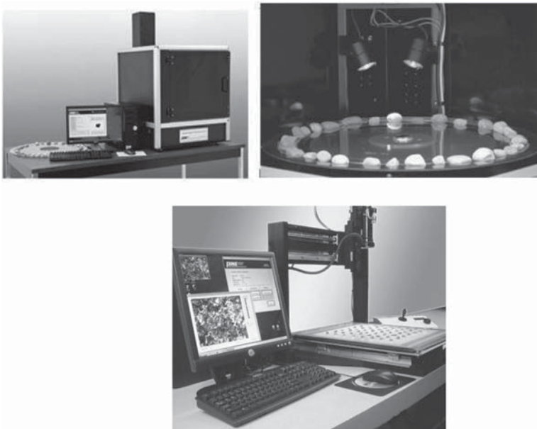
FIGURE 8.10 Automated aggregate imaging system. (Courtesy Pine Instruments, Grove City, PA.)
