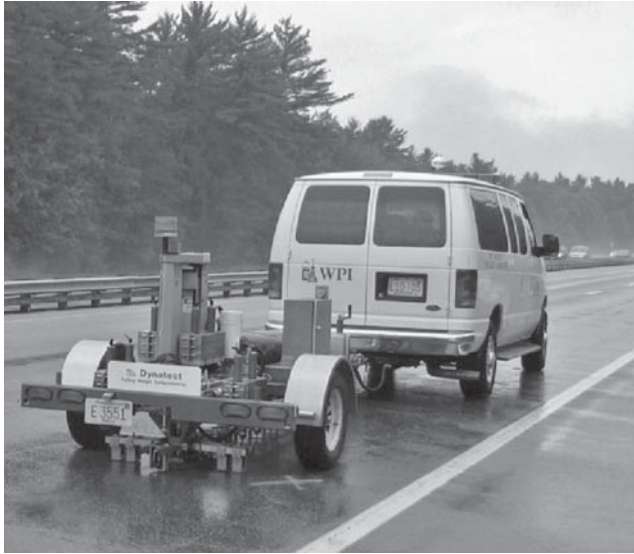
FIGURE 18.4 Falling weight deflectometer.
