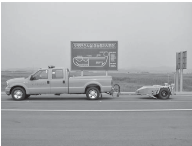
FIGURE 18.5 Skid tester. (Courtesy of David Morrow, Dynatest Consulting Inc., Ventura, CA.)
