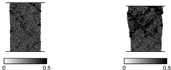
Figure 8.4: Plot of deformed sample at (a) 5.5% and (b) 12% for biaxial simulation of 2,376 unbonded disks, confined with stress-controlled membrane. Shading illustrates magnitude of disk rotation in radians
