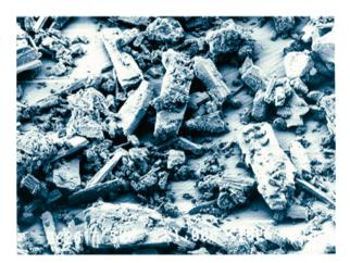
**Fig. 3** Scanning electron micrograph: micronized HAR wollastonite flour (magnification 1:1,000)
