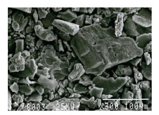
**Figure 6** SEM of calcined clay (kaolin)
