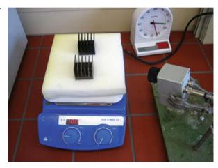
isolated versus the surroundings. Figure 5 shows the setup with the EP/alumosilicate heat sink at the front.
